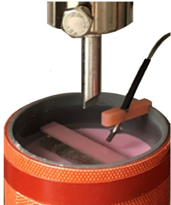
Fig. 3. Set-up for the 3-point FS measurement in 37 °C tempered water.
