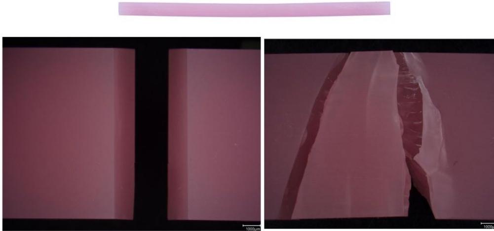
Fig. 5. Fracture types a. deformation of the specimen, b. 90° fracture between the printing layers resulting in two fracture pieces, c. complex fracture into \geq 3 parts.
