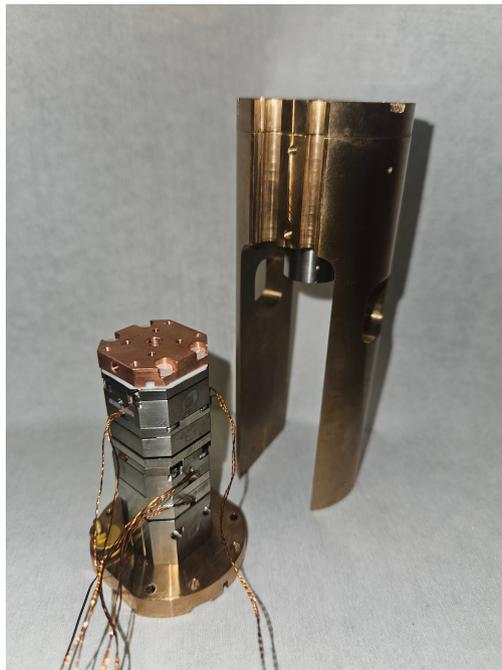
Figure 3.4: Experiment cage made of non-magnetic phosphor bronze with a stack of piezo stepping and scanning positioners from Attocube systems (ANP101 and ANS100). The top plate on the stack is made of oxygen-free copper and it is thermally isolated from the positioners by a teflon spacer. The sample holder is then located on top of this plate and connected to the cold stage by flexible copper braids, allowing for simultaneous cooling and positioning.
