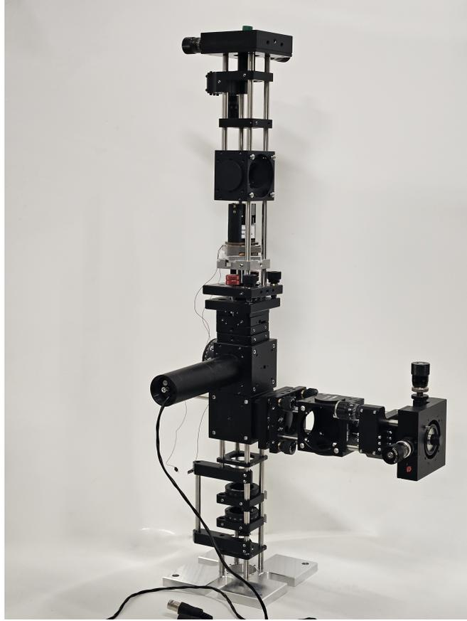
Figure 3.6: Photograph of the assembled microscope head that was used together with the dilution refrigerator setup.
