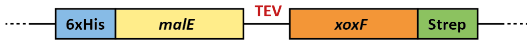
Fig. S1. N -terminal maltose-binding protein ( malE ) construct. Final construct for production of the maltose binding protein-XoxF-MDH fusion with additional Strep -tag, His-tag and protease cleavage site.
