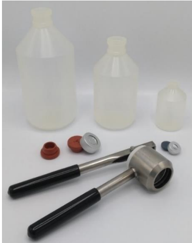
Fig. S10. Plastic cultivation flasks (injection or infusion bottles) for growth experiments of strain SolV with Lns and Ans. Flasks: polypropylene, volume 1000 mL, 500 mL and 100 mL; Stoppers: bromobutyl rubber, Ø 32 mm (for 1000 mL and 500 mL) or Ø 20 mm (100 mL); Caps: aluminum.
