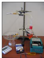
Figure 2: Experimental set-up for the production of cigarette smoke extract (CSE) (left) and conditions of cell culture (right)
