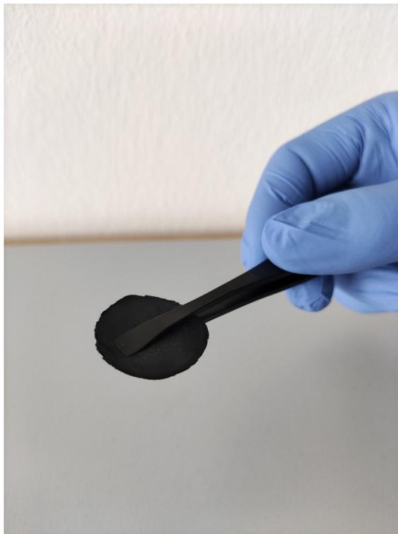
**Figure 7.10:** Photograph of a freestanding ATO/C/rGO electrode showing its mechanical stability.
