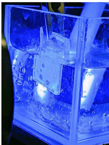
**Figure 5.12:** Oxygen bubble formation on the electrode during photoelectrochemistry.
