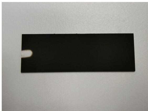
**Figure 3.6:** Photograph of as-deposited carbon soot on soda-lime glass (SLG).
