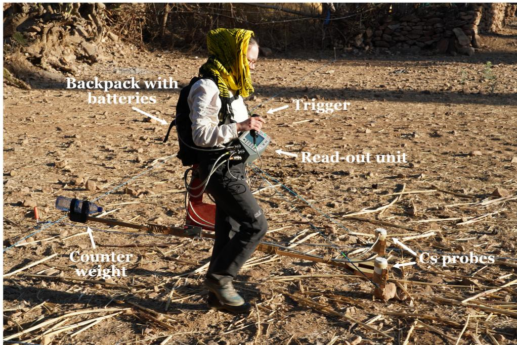
**Figure 2.3:** *Prospecting of the Geometric's instrument. The Caesium probes are fixed on a wooden frame to move the whole setup around 30 cm above the ground. The probes are connected to the read-out unit, powered by the batteries carried in the backpack. A water bottle is used as a counterweight.*
