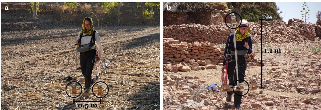
**Figure 2.6:** a) Measurement with the Geometrics magnetometer. The sensors are mounted at a horizontal distance of 0.5 m on the frame. Both sensors are moved parallel to the survey direction. This setup is called duo-sensor configuration or horizontal gradiometer mode. The processing of the data determines which of the two it is. b) Survey in vertical gradiometer mode with both sensors mounted on top of each other.
