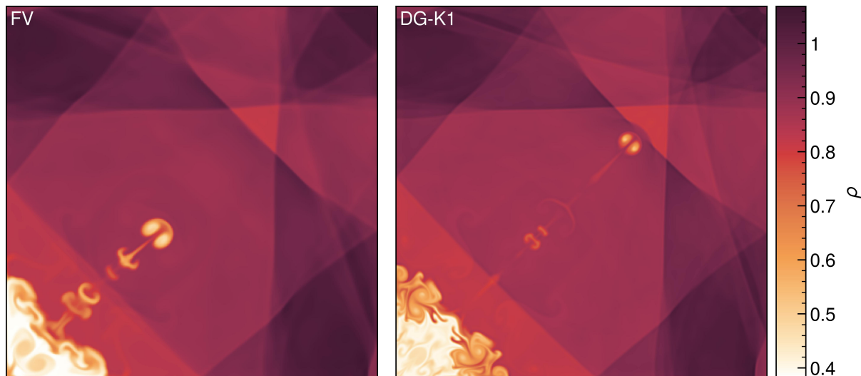
Figure 3.2: Density field of the Liska & Wendroff (2003) implosion test at time t = 2.5 , simulated with 400 \times 400 cells either with DG at order k = 1 (right panel), or with a finite volume scheme (left panel). Both methods describe the fluid with linear functions inside cells. The initial conditions contain a region of strongly reduced density and pressure in the lower left corner. This launches a shock towards the origin which reflects at the reflecting boundaries of the domain. The interaction of the shocks at the corner and the diagonal produces a jet of dense gas along the diagonal direction. The test is very sensitive to numerical diffusion, which tends to limit the length of the diagonal jet. As our results demonstrate, our DG scheme is not only capable of capturing the strong shock interactions while accurately maintaining the symmetry of the system, it also shows clearly less numerical diffusion than the equivalent finite volume scheme.
