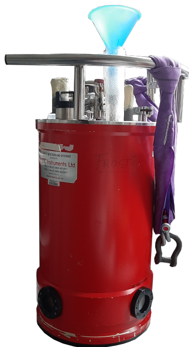
Figure 1.20: The liquid-He-cooled InSb Hot Electron Bolometer (HEB) detector used for the measurements with the CASAC setup. The black circular components on the bottom of the detector are where the radiation gets in and out of the bolometer. The blue funnel corresponds to the liquid N 2 inlet.
