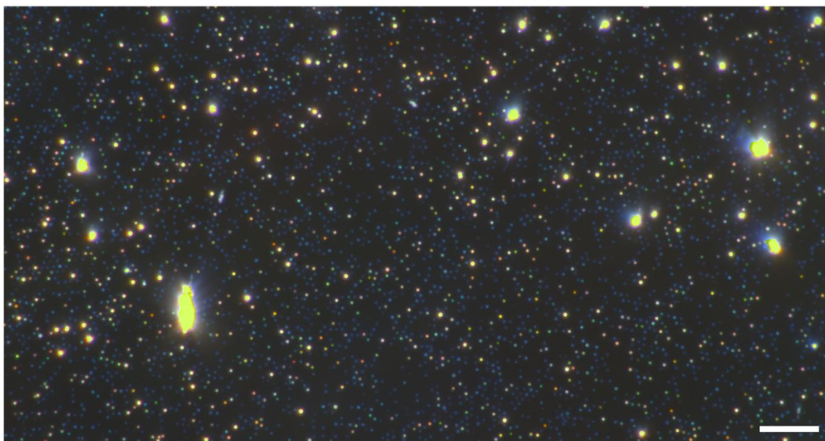
Figure S32. DFM image of a PUF with 1 \mu\text{m} spacing. Particles used – AgNS @ 0.6 OD. NPP was performed with AgNS directly without a DOP step. A pattern of scattering spots is visible, showing that it is possible to achieve placement of nanoparticles without DNA Origami. However, scattering spot density is low and the hue response is largely monochromatic, with a majority of the scattering spots showing blue hues similar to individual AgNS. Scale bar, 10 \mu\text{m} .
