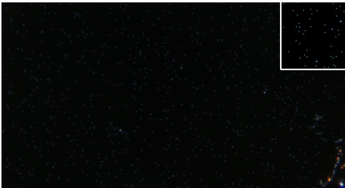
Figure S30. DFM images of AuNS deposited on glass slides recorded at 100x magnification. Insets: Magnified view with enhanced contrast to ease visualization.
