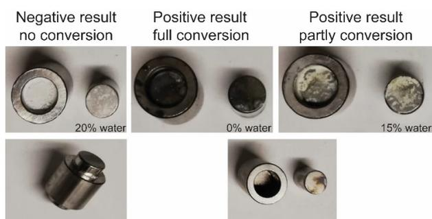
**Figure 6.** Fallhammer specimen holder after various tests. Negative tests remain closed (bottom left) positive tests are usually opened through the detonation (bottom right).
