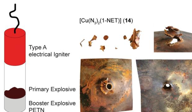
Fig. 15 Left: Initiation test setup without a copper witness plate. Right: Result of the initiation experiment of compound **14** toward PETN.
