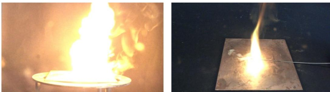
**Figure S40.** Deflagration of the picrate complex **20** during hot plate test (left) and hot needle tests (right).
