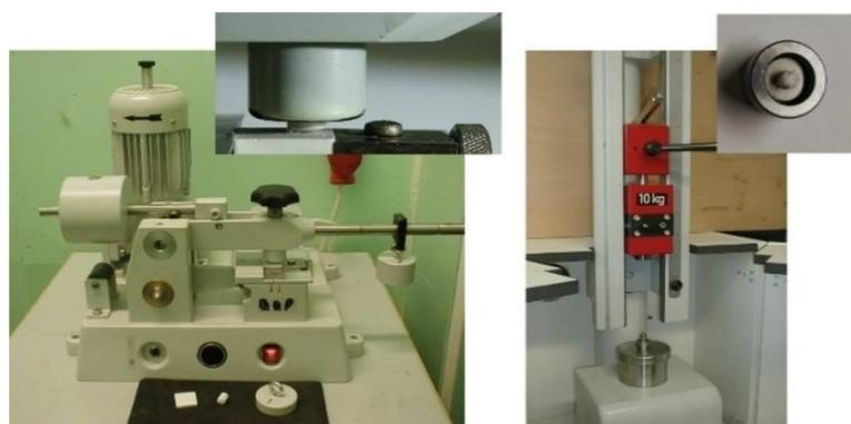
**Figure 7** Mechanical sensitivity measurement with BAM friction tester (left) and impact tester (right).
