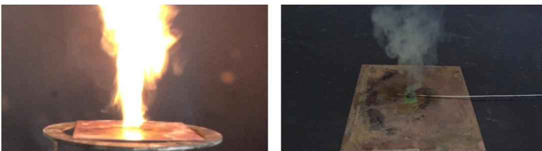
**Figure S36.** Deflagration of the picrate complex **17** during hot plate test (left) and decomposition during hot needle test (right).
