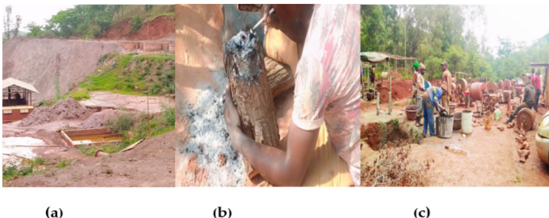
Figure 3. Chemical pollution in the workplace: (a) chemical contamination: cyanide leaching from mercury-containing tailings and dust from tailings, Shurugwi 2020; (b) open amalgam burning, Kadoma 2020; (c) fuel emissions from fuel-powered machinery and dust from mercury-containing tailings, Shurugwi 2020.
