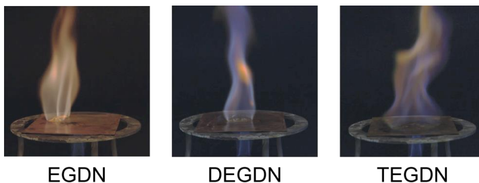
Figure 12. Hot-plate test of the investigated ethylene glycol dinitrates.
