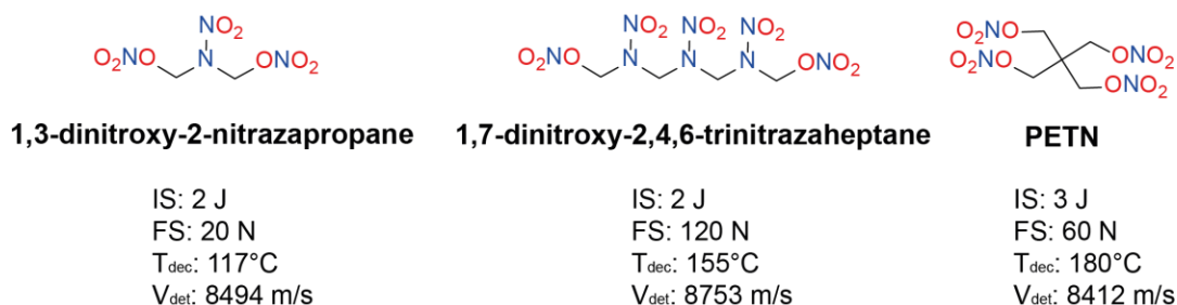
Figure 7. Compared properties of 1,3-dinitroxy-2-nitrazapropane, 1,7-dinitroxy-2,4,6-trinitrazaheptane and PETN.
