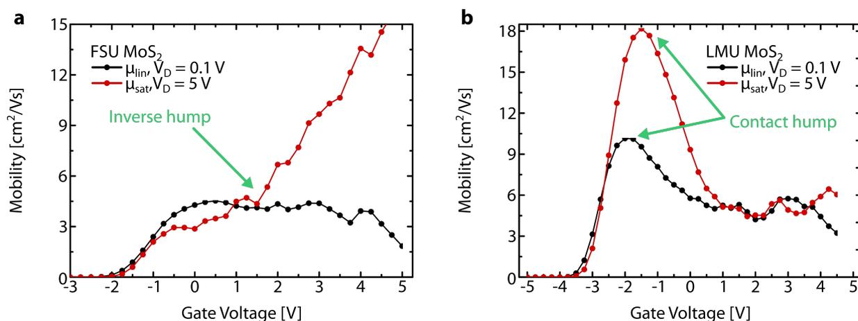
**Figure 4.11:** Mobility characteristics of **a** FSU MoS<sub>2</sub> TFTs, and **b** LMU MoS<sub>2</sub> TFTs for low and high drain biases. FSU and LMU indicates the provider of the MoS<sub>2</sub> crystals.
