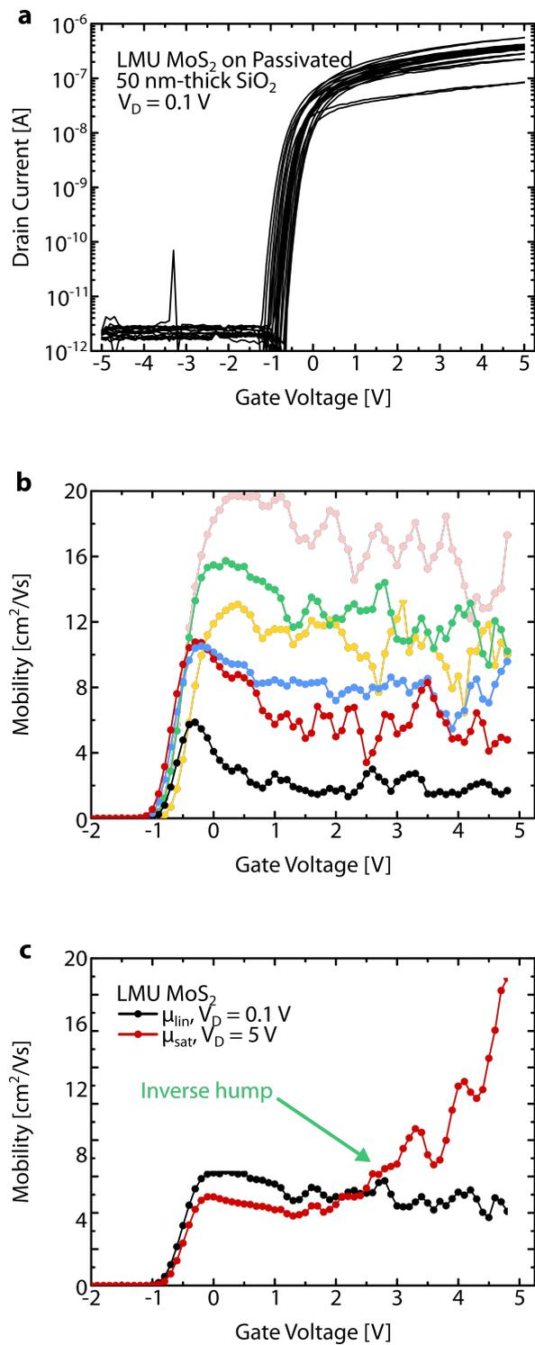
**Figure 4.12:** Characteristics of LMU MoS<sub>2</sub> TFTs on passivated 50 nm-thick oxide. **a** Transfer curves of 10 LMU MoS<sub>2</sub> transistors on a semi-logarithmic scale. **b** Linear mobility characteristics of the selected transistors. **c** Mobility characteristics of MoS<sub>2</sub> TFT under 0.1 V and 5 V drain bias.
