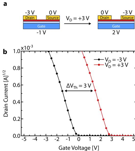
**Figure 2.18:** Illustration and investigation of the polarity-dependent saturation current characteristics of the DNTT TFT. **a** Illustration of the proper (left) and the equivalent (right) circuit depending on the drain bias polarity. Red and light blue regions represent the semiconductor and the gate oxide, respectively. **b** Saturation current characteristics of DNTT TFT under positive and negative drain bias. Threshold voltage shift is indicated as  $\Delta V_{Th}$ .
