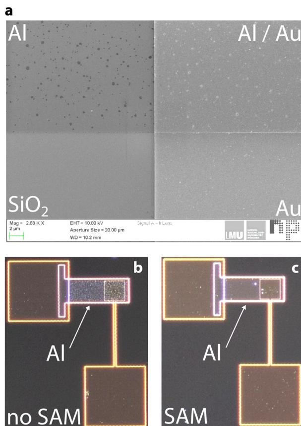
**Figure 5.11:** Plasma-associated PMMA contamination on the aluminum film. **a** SEM image of the capacitor intersection. Optical microscopy images of the **b** untreated, and **c** SAM-passivated oxides for capacitor test structures.
