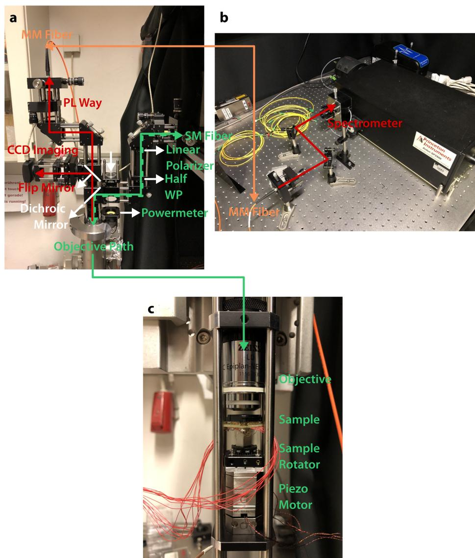
**Figure D.6:** The new microscope. **a** Optical construction of the microscope. **b** PL path of the microscope. **c** Position of the objective and the sample.
