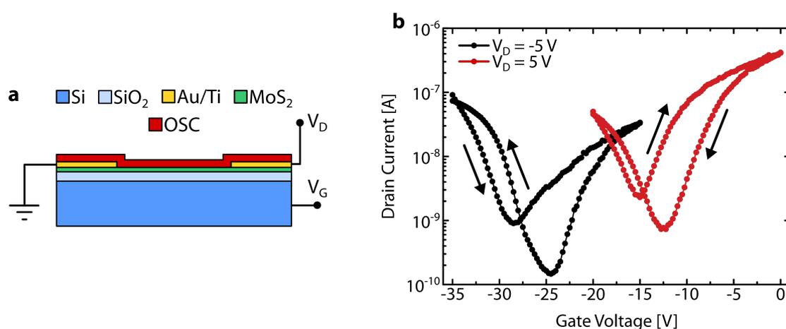
**Figure 3.14:** Characteristics of ambipolar MoS<sub>2</sub>/DNTT transistors on 90 nm-thick silicon oxide for  $\pm 5$  V drain voltage. The arrows indicate the sweep directions.
