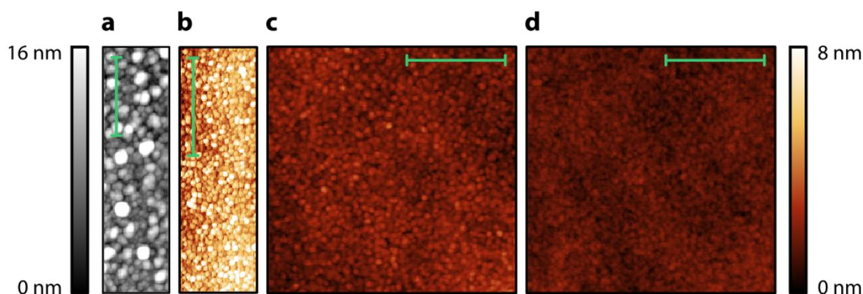
**Figure 5.7:** Determination of the roughness of 30 nm-thick aluminum films by AFM. **a** Electron-beam evaporated, and **b** thermally evaporated aluminum films. Thermally evaporated aluminum film **c** after 1 min, and **d** after 5 min plasma oxidation. Scale bars are 400 nm for all micrographs.
