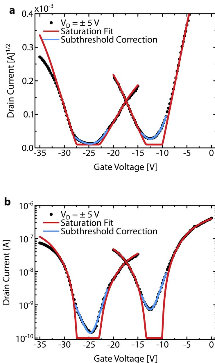
**Figure 3.17:** Revealed saturation and subthreshold regions of ambipolar MoS<sub>2</sub>/DNTT transistor for  $\pm 5$  V drain biases. Transfer curves of the ambipolar transistor on **a** square-root and on **b** semi-logarithmic scales in BW sweep. The red and blue solid lines represent saturation and subthreshold regions, respectively.
