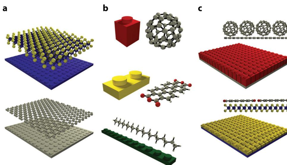
**Figure 1.4:** Illustration of inorganic nanosheet stacking with organic molecules for building van der Waals heterostructures. **a** Inorganic nanosheets. The blue and gray blocks represent  $\text{MoS}_2$  and graphene, respectively. **b** Organic 0D and 1D small molecules. The red and yellow blocks represent buckminsterfullerene and perylene-tetracarboxylic dianhydride, and the green block represents docosane. **c** Organic/inorganic van der Waals heterostructures. Adapted from [18].
