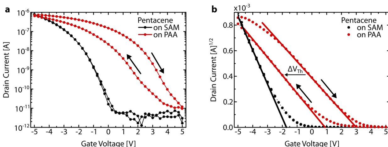
**Figure 3.10:** Characteristics of TC as-evaporated pentacene TFTs on SAM and PAA. Transfer curves of pentacene TFTs on **a** semi-logarithmic and **b** square-root scales. The black and red solid lines represent the extrapolations of saturation currents. The saturation current characteristics are for BW sweep direction.
