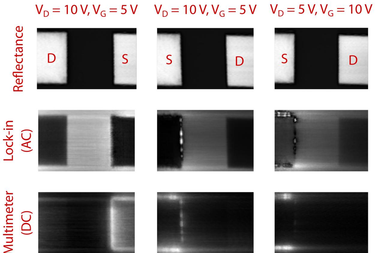
**Figure B.9:** Reflectance, AC (measured by lock-in amplifier) and DC (measured by digital multimeter) current photocurrent micrographs of MoS<sub>2</sub> TFTs with different bias and contact conditions. S and D represent source and drain, respectively. The diode laser was operated at 2 kHz with a laser power of  $0.4 \mu\text{Wcm}^{-2}$ .
