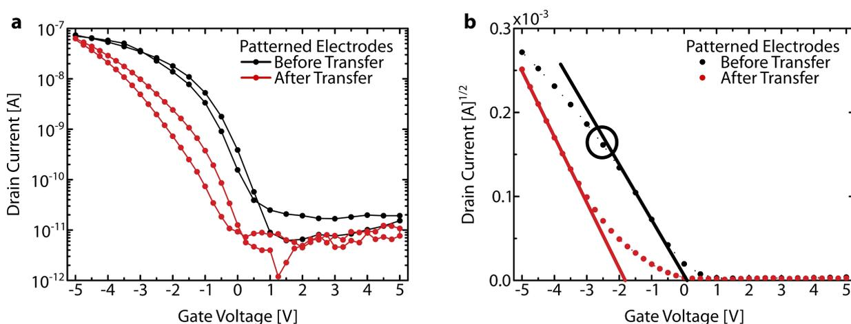
**Figure 3.13:** Characteristics of TC transferred pentacene TFTs with contact patterning before or after transfer. Transfer curves of pentacene TFTs on **a** semi-logarithmic and **b** square-root scales. The black, and red solid lines represent the extrapolations of saturation current. The black circle indicates the saturation-to-linear transition point. The saturation current characteristics are for BW sweep direction.
