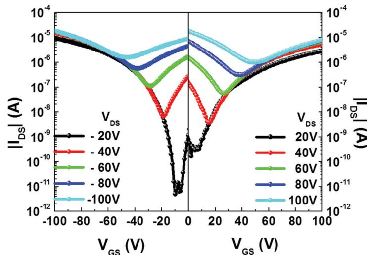
**Figure 2.19:** Drain bias-dependent ambipolar current behavior in QBS TFT. The left and right sides of the graph represent negative and positive drain biases, respectively. Taken from [62].
