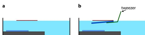
**Figure 3.7:** Illustrations of nanosheet pick-up. **a** The free floating nanosheet in beaker. **b** The nanosheet pick-up.
