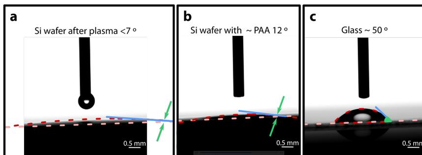
**Figure B.2:** Contact angle measurements of the substrate, PAA, and the glass carrier.
