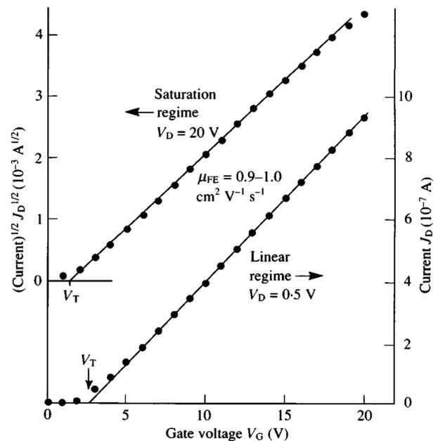
**Figure 2.11:** Determination of linear and saturation regions in a-Si:H TFT. The transfer curve on the square-root and linear scales are represented on the left and right y-axes, respectively. The estimated threshold voltages are indicated by  $V_T$ . Adapted from [55].
