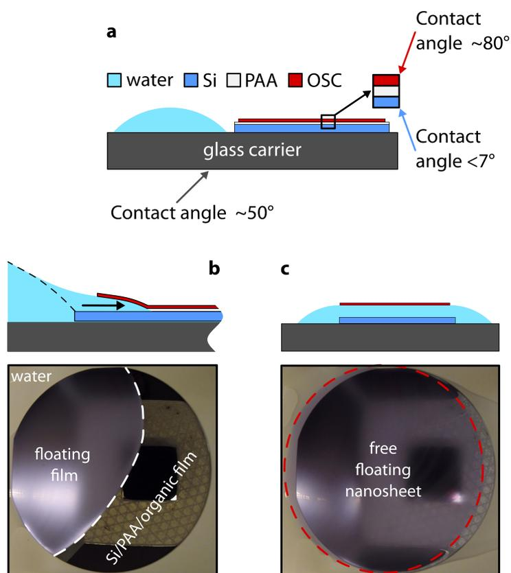
**Figure 3.6:** Nanosheet release by side injection. **a** Illustration of the wetting geometry before contact. **b** Illustration and picture of the release process during dissolving. The white dashed line indicates the border of the floating nanosheet. The black arrow represents the advancing direction. **c** Illustration and picture of the free floating nanosheet. The red dashed circle indicates the border of the free floating nanosheet.
