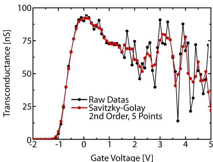
**Figure B.11:** Comparison of with and without Savitzky-Golay filtering for transconductance of MoS<sub>2</sub> TFT.
