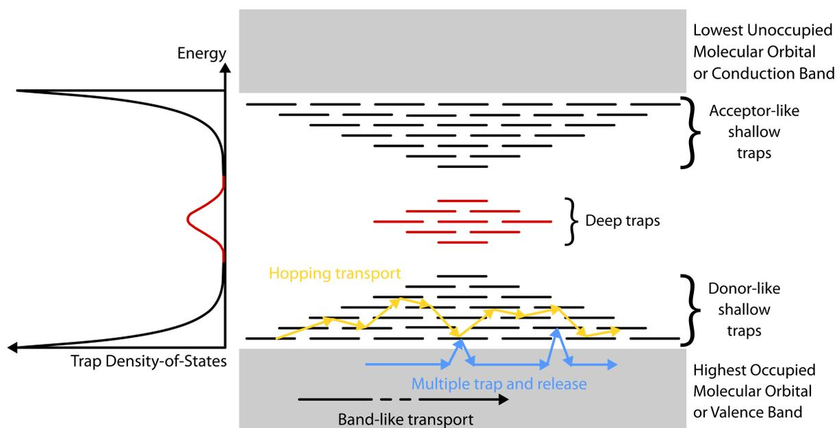
Figure 2.5: Illustration of charge transport models in semiconductors. Adapted from [49].
