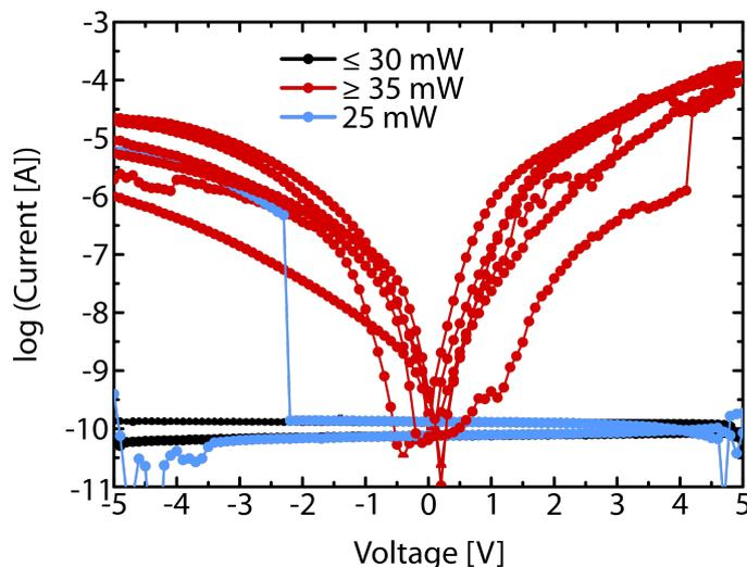
**Figure B.8:** Leakage current measurements of Si/SiO<sub>2</sub>/Ti/Au capacitors as a parameter of bonding power.
