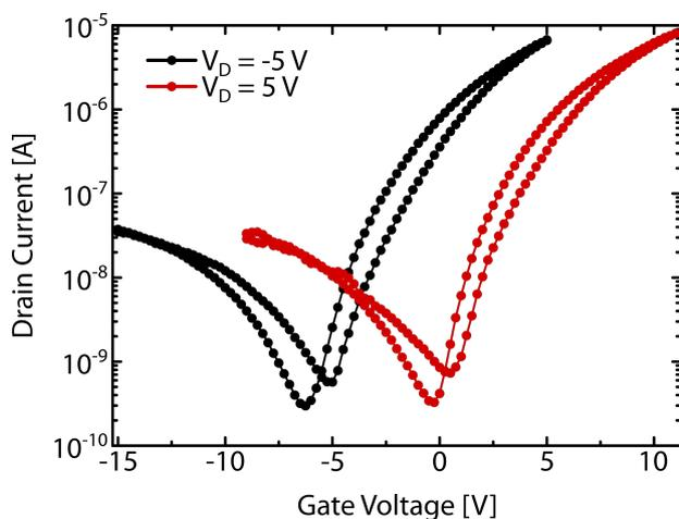
**Figure 4.4:** Characteristics of ambipolar  $\text{MoS}_2$ /DNTT transistors on passivated 90 nm-thick oxide for  $\pm 5$  V drain voltage.
