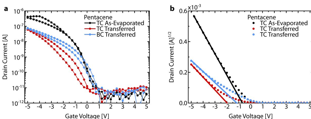
**Figure 3.11:** Characteristics of transferred pentacene TFTs in various configurations. Transfer curves of benchmark (TC as-evaporated) pentacene TFT and TC/BC transferred pentacene TFTs on **a** semi-logarithmic and **b** square-root scales. The black, red, and blue solid lines represent the extrapolations of saturation currents. The saturation current characteristics are for BW sweep direction.
