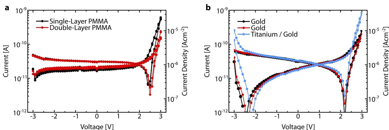
**Figure 5.12:** Leakage current characteristics of the capacitors with plasma-enhanced aluminum oxide as dielectric. Impact of **a** resist undercut, and **b** contact material.
