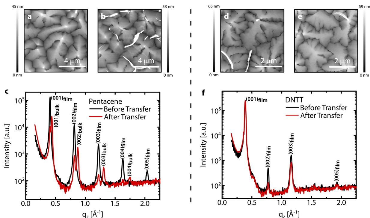
**Figure 3.9:** Morphology and crystallinity of 50 nm-thick pentacene and DNTT nanosheets before and after transfer. Atomic force micrographs of pentacene film **a** before and **b** after transfer. **c** X-ray diffraction measurements on pentacene film before and after transfer. Film and bulk indicate the packing motif of pentacene. Atomic force micrographs of DNTT film **d** before and **e** after transfer. **f** X-ray diffraction measurements on DNTT film before and after transfer.
