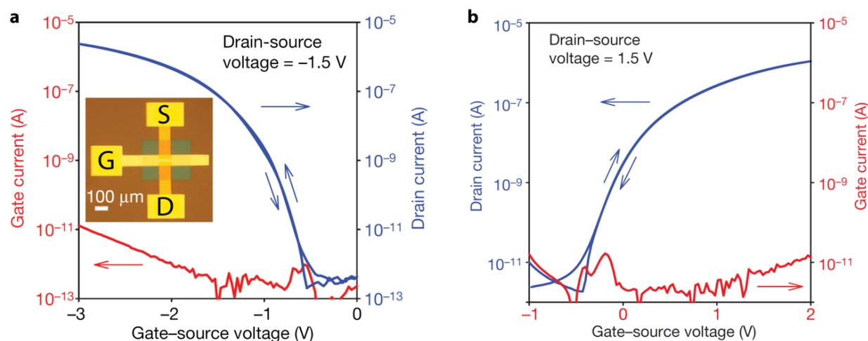
**Figure 5.2:** Low-voltage pentacene and  $\text{F}_{16}\text{CuPc}$  transistors on passivated plasma-enhanced aluminum oxide. **a** Drain and gate currents of pentacene TFT on a semi-logarithmic scale. Inset represents the optical microscopy image of the transistor. **b** Drain and gate currents of  $\text{F}_{16}\text{CuPc}$  TFT on a semi-logarithmic scale. Adapted from [39].
