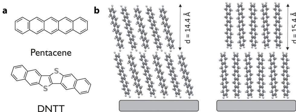
**Figure 2.2:** Molecular structure and packing motifs of small molecules. **a** Molecular structure of pentacene and DNNT. **b** Packing motifs of pentacene molecules. Left: Campbell bulk-phase with a molecular tilt of  $21^\circ$ . Right: Thin-film phase with a molecular tilt of  $3^\circ$ . The length of the pentacene molecule is  $15.5 \text{ \AA}$ . Adapted from [37, 38].
