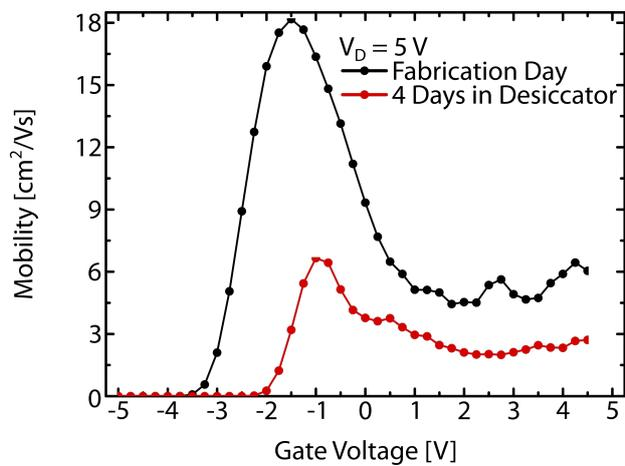
**Figure B.5:** Effect of ambient conditions on the mobility of the TFTs over days.
