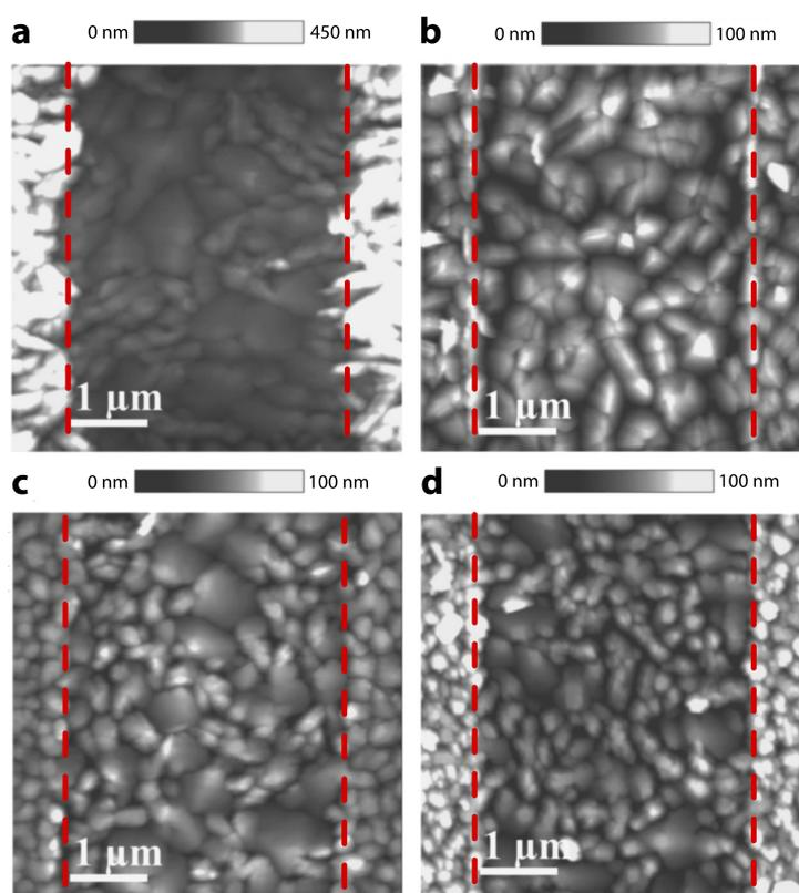
**Figure 3.1:** Crystallization of pentacene on untreated and SAM passivated gold revealed by AFM. **a** untreated gold, **b** C<sub>7</sub>-SAM passivated gold, **c** C<sub>12</sub>-SAM passivated gold, and **d** AnT-SAM passivated gold. Red dashed lines indicate gold/oxide intersections. Adapted from [63].
