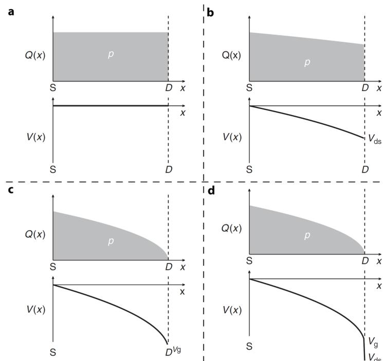
**Figure 2.8:** Distribution of field-effect charge density  $Q(x)$  and channel potential  $V(x)$  along the channel as a parameter of drain bias for p-channel TFT. **a**  $V_D = 0$  V, **b**  $V_D \ll V_G$ , **c**  $V_D = V_G$ , and **d**  $V_D > V_G$ . S and D indicate source and drain electrodes, respectively. Adapted from [50].
