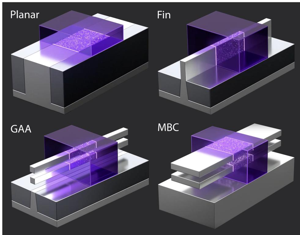
**Figure 1.1:** “Evolution” of the MOSFET: Planar, fin, gate-all-around (GAA), and multiple-bridge-channel field-effect transistors. The purple region represents the gate oxide, and the dotted region represents the transistor channel. Adapted from [5].
