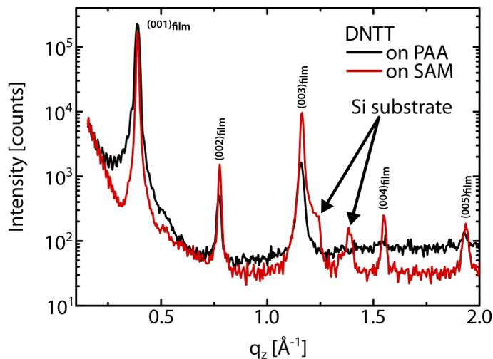
Figure B.12: XRD of as-evaporated polycrystalline DNTT films on PAA and SAM.
