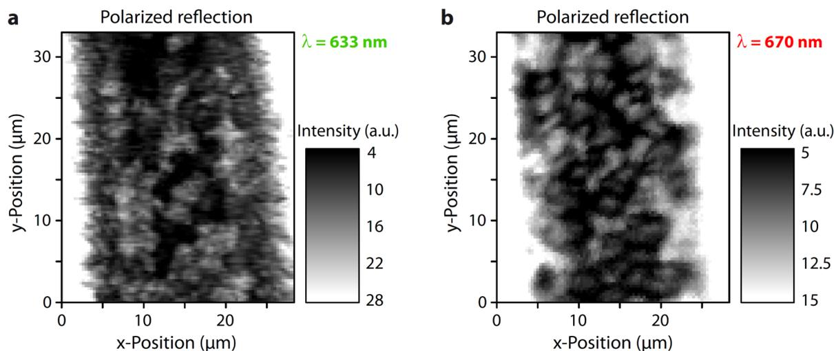
**Figure D.2:** Davydov splitting in pentacene thin film as a function of laser wavelength, measured by C. Westermeier. Adapted from [102].
