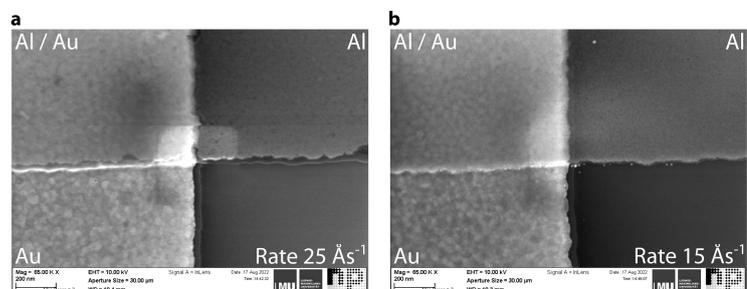
**Figure 5.10:** Effect of aluminum evaporation rate on the edge quality of the gate stack. **a**  $25 \text{ \AA s}^{-1}$ . **b**  $15 \text{ \AA s}^{-1}$ .
