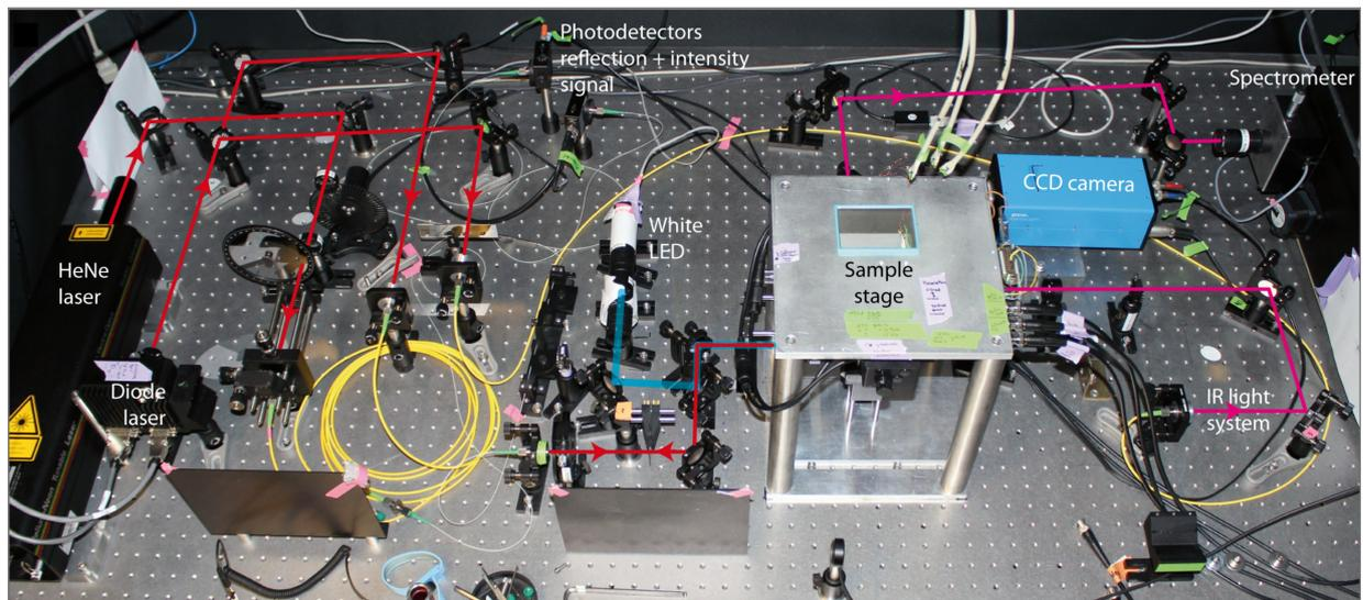
Figure D.1: The former microscope setup. Adapted from [102].
