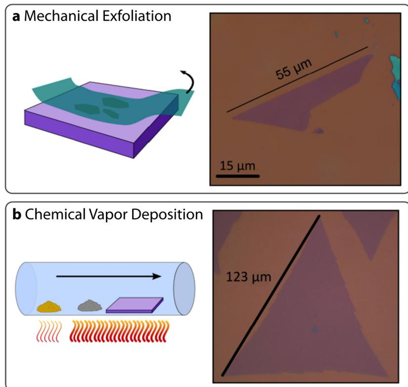
**Figure 2.4:** Top-down and bottom-up deposition methods of  $\text{MoS}_2$  crystals. **a** Optical microscopy image of  $\text{MoS}_2$  crystals deposited by mechanical exfoliation. The blue sheet represents the adhesive tape. **b** Optical microscopy image of  $\text{MoS}_2$  crystals deposited by CVD method. An inert gas carries the heated precursors (black arrow) for deposition on the substrate. Adapted from [47, 48].
