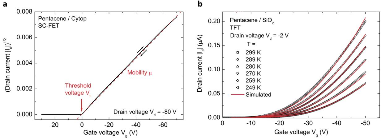
**Figure 2.12:** Transistor characteristics of pentacene single crystal and thin-film transistors. **a** Square-root plot of the transfer curve of pentacene single-crystal FET on CYTOP dielectric at room temperature. The red dashed line indicates the extrapolation of saturation current. **b** Linear plot of the transfer curve of pentacene TFT on SiO<sub>2</sub> for various temperatures. Adapted from [56].
