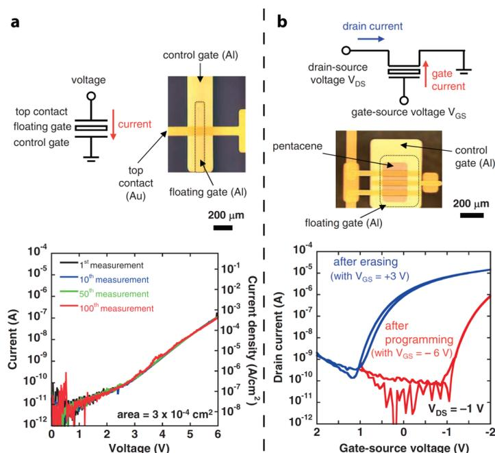
**Figure 5.3:** Characteristics of the floating-gate memory transistors. **a** Top: Illustration and the optical microscopy image of the floating-gate capacitor. Bottom: Leakage current characteristics of the floating-gate capacitor over 100 sweep cycles. **b** Top: Illustration and the optical microscopy image of the floating-gate transistor. Bottom: Characteristics of the floating-gate transistor. Programming and erasing read-outs exhibited a memory window of 2 V. Adapted from [87].
