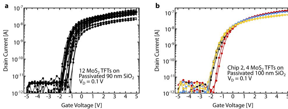
**Figure B.6:** Reproducibility of MoS<sub>2</sub> TFTs on COC-passivated oxide. Semi-logarithmic plot of the transfer curve of a 12 MoS<sub>2</sub> TFTs on passivated 90 nm oxide (Chip 1), b 4 MoS<sub>2</sub> TFTs on passivated 100 nm oxide (Chip 2).
