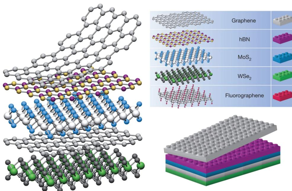
**Figure 1.3:** Illustration of inorganic nanosheet stacking for building van der Waals heterostructures. Taken from [11].
