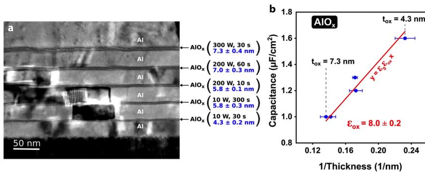
**Figure 5.5:** Determination of the thickness of plasma-enhanced aluminum oxides for various plasma parameters. **a** Cross section TEM image of several gate stacks for various plasma powers and duration. **b** Capacitance-thickness curve of the plasma-enhanced aluminum oxide for the determination of relative dielectric constant. Adapted from [89].
