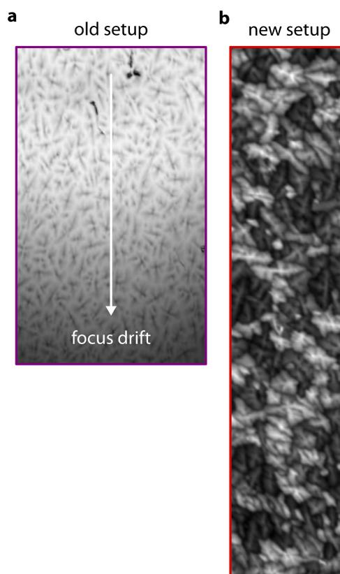
**Figure D.5:** Change in the reflection intensity during the mapping. **a** 405 nm former version. **b** 635 nm new version.
