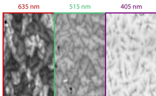
**Figure D.4:** Reflection micrographs of pentacene thin film under 635 nm, 515 nm and 405 nm laser wavelengths.
