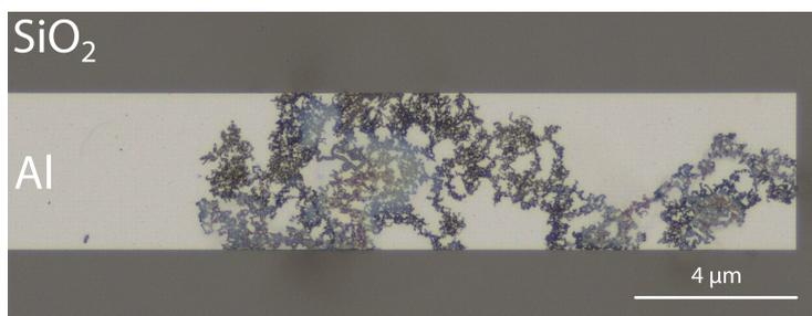
**Figure 5.8:** Chlorine-associated aluminum corrosion after plasma oxidation.
