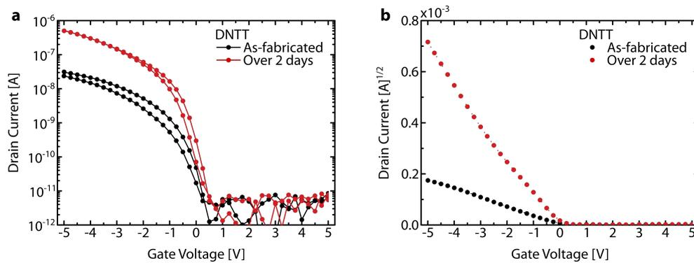
**Figure B.4:** The comparison of transistor characteristics of BC transferred DNTT TFTs as-fabricated and over days. **a** Semi-logarithmic and **b** square-root plots of transfer curves of transferred DNTT TFTs measured as-fabricated (black dotted line) and over the weekend (red dotted line).
