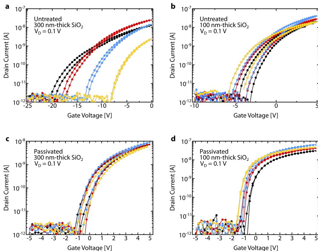
**Figure 4.7:** Characteristics of MoS<sub>2</sub> TFTs on untreated and passivated oxides as a parameter of oxide thickness under  $V_D = 0.1$  V. Semi-logarithmic plot of the transfer curve of MoS<sub>2</sub> TFTs on **a** untreated 300 nm-thick SiO<sub>2</sub>, **b** untreated 100 nm-thick SiO<sub>2</sub>, **c** passivated 300 nm-thick SiO<sub>2</sub>, and **d** passivated 100 nm-thick SiO<sub>2</sub>.
