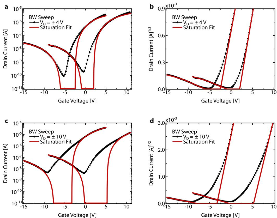
**Figure 4.6:** Revealed saturation regions of ambipolar  $\text{MoS}_2/\text{DNTT}$  transistors on passivated oxide under high drain biases. Transfer curve of the ambipolar transistors on passivated 90 nm-thick oxide for drain voltages of  $\pm 4$  V and  $\pm 10$  V, on **a, c** semi-logarithmic and **b, d** square-root scales. The red solid lines represent the electron and hole saturation regions.
