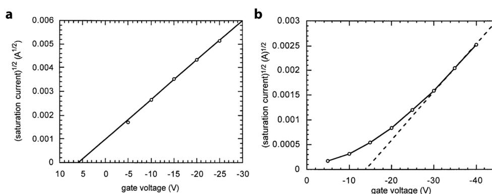
**Figure 2.10:** Characteristics of DH6T TFTs in ambient and in vacuum. **a** DH6T TFT kept and measured in ambient. The solid line indicates the extrapolation of the saturation current. **b** DH6T TFT kept and measured in vacuum. The dashed line indicates the extrapolation of the saturation current. Adapted from [54].
