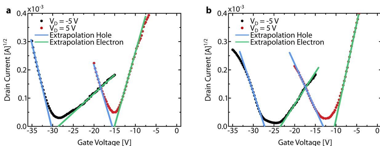
**Figure 3.15:** Transfer curves of ambipolar MoS<sub>2</sub>/DNTT transistors on a square-root scale for  $\pm 5$  V drain voltage in **a** FW and **b** BW sweeps.
