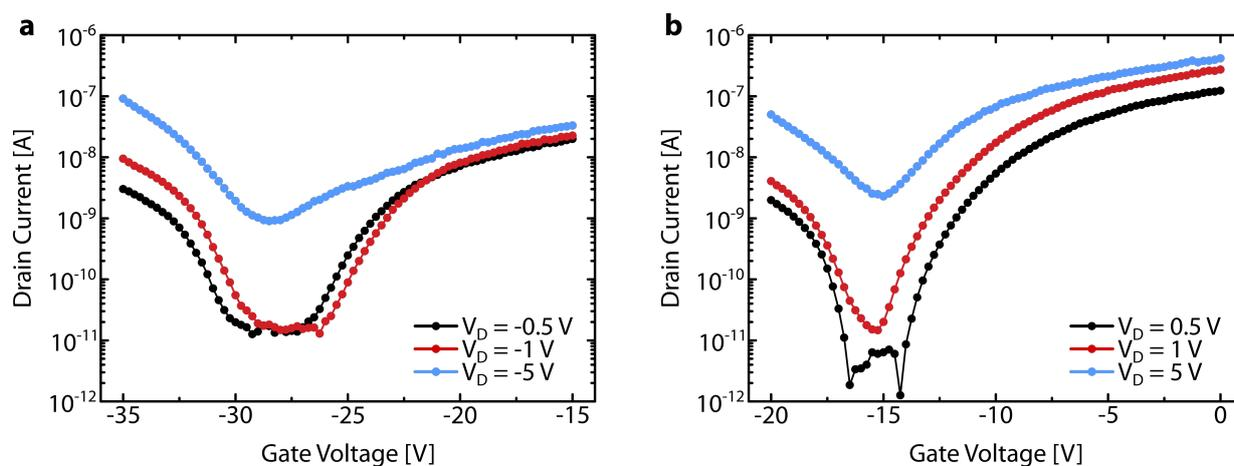
**Figure 3.16:** Transfer curves of ambipolar  $\text{MoS}_2/\text{DNTT}$  transistors on a semi-logarithmic scale under various **a** negative and **b** positive drain biases in FW sweep.
