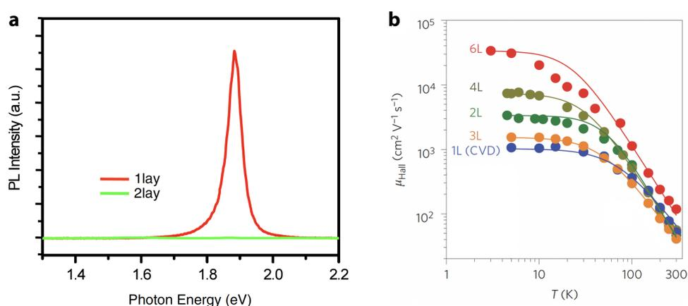
**Figure 2.3:** Layer number dependent **a** photoluminescence and **b** Hall mobility of  $\text{MoS}_2$  crystals. Adapted from [14, 40].
