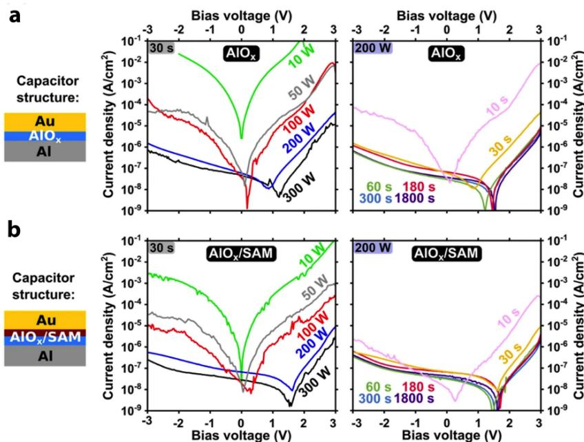
**Figure 5.6:** Leakage current characteristics of untreated and SAM-passivated plasma-enhanced aluminum oxide for various plasma parameters for **a** untreated oxide, and **b** SAM-passivated oxide. Adapted from [89].
