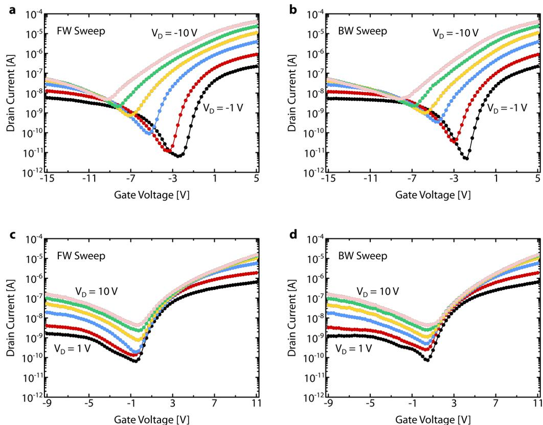
**Figure 4.5:** Semi-logarithmic plot of transfer curves of MoS<sub>2</sub>/DNTT ambipolar transistors on passivated 90 nm-thick oxide under various drain biases for **a** FW and **b** BW sweep directions for negative drain voltages. **c** FW and **d** BW sweep directions for positive drain voltages.
