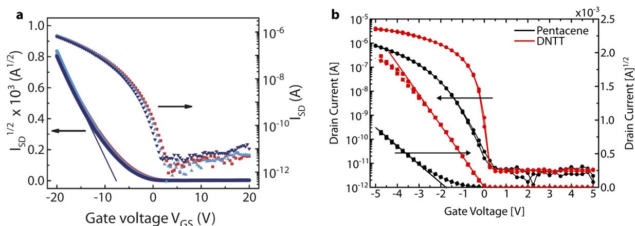
**Figure C.1:** Transistor characteristics of organic TFTs with previous and the new oxide stack. **a** Pentacene TFT on SiO<sub>2</sub>/COC gate stack. **b** Pentacene and DNTT TFTs on Al<sub>2</sub>O<sub>3</sub>/SAM gate stack.
