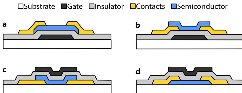
Figure 2.7: Thin-film transistor configurations. **a** Bottom-gate top-contact, **b** bottom-gate bottom-contact, **c** top-gate bottom-contact, **d** top-gate top contact.
