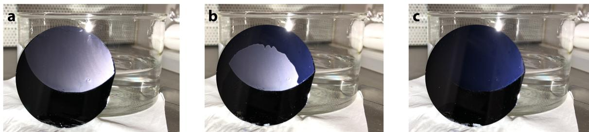
**Figure 3.8:** Pictures of organic nanosheets during lamination. **a** After pick-up, **b** half-laminated, and **c** completely laminated.
