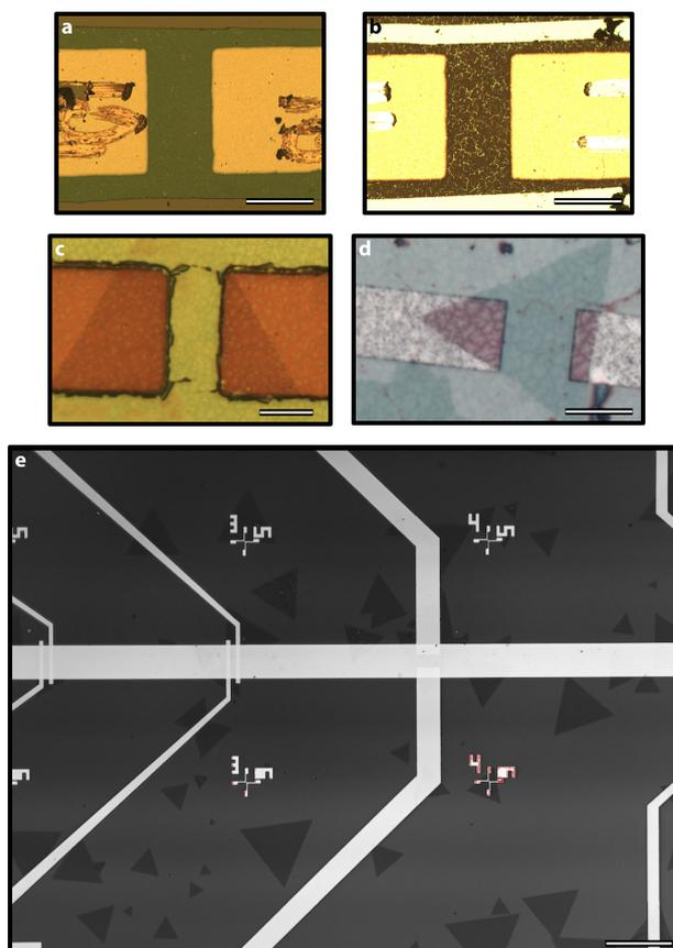
**Figure B.3:** Typical device images of unipolar/ambipolar nanosheet TFTs. **a** Unipolar DNTT (scalebar is 100  $\mu\text{m}$ ), **b** unipolar pentacene (scalebar is 100  $\mu\text{m}$ ), **c** ambipolar  $\text{MoS}_2$ /DNTT photolithographically patterned, **d** ambipolar  $\text{MoS}_2$ /DNTT electron beam lithographically patterned, and **e** unipolar  $\text{MoS}_2$  on plasma-enhanced oxide. Scale bars are 100  $\mu\text{m}$  for **a** and **b**, 10  $\mu\text{m}$  for the others.
