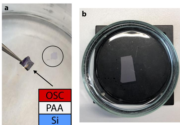
**Figure 3.4:** Nanosheet release by immersion to water. **a** Picture of the sample during immersion. Free floating nanosheet (approximately 16 mm<sup>2</sup>) is encircled by a black circle. The inset represents the illustration of the substrate (not to scale). **b** Free floating nanosheet in sizes of 7 mm x 15 mm.
