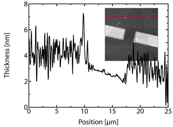
**Figure 4.2:** Determination of surface roughness of a COC-encapsulated MoS<sub>2</sub> transistor by AFM. The red solid line represents the line profile.
