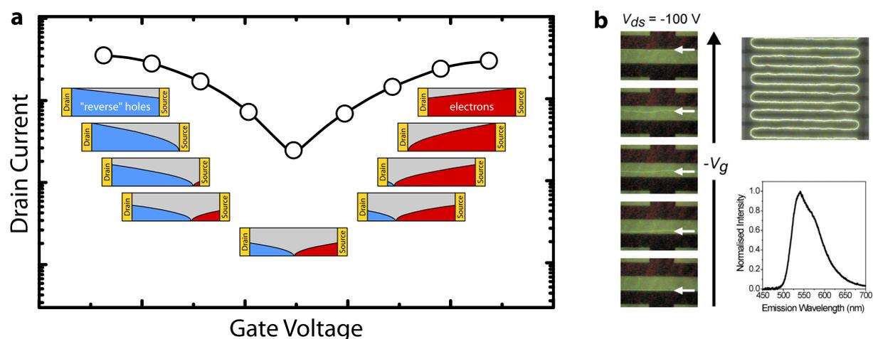
**Figure 2.17:** Illustration and investigation of charge transport in ambipolar transistors as a function of gate bias. **a** Illustration of gate bias-dependent charge distribution in an ambipolar semiconductor. **b** F8BT light-emitting field-effect transistor. The white arrow represents the recombination zone as a parameter of gate bias. Adapted from [25].
