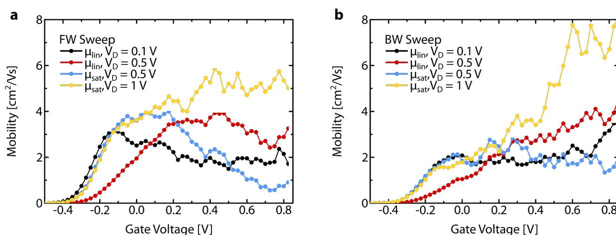
**Figure 5.16:** Mobility characteristics of low voltage MoS<sub>2</sub> TFTs on plasma-enhanced gate stack for various drain biases.
