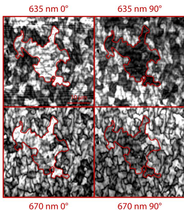
**Figure D.3:** High resolution Davydov splitting in pentacene thin film as a function of laser wavelength and polarization.
