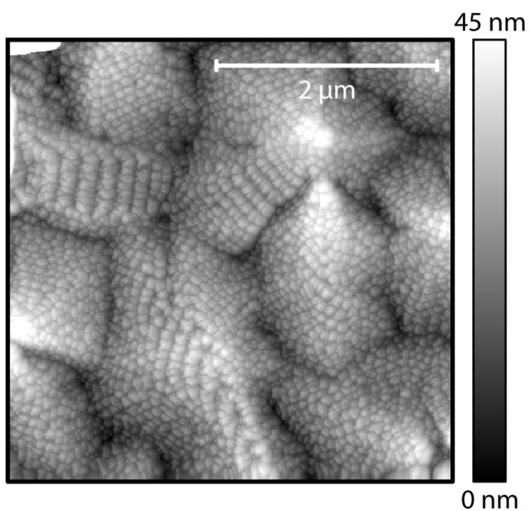
**Figure B.1:** Transferable pentacene/C<sub>60</sub> heterojunction.
