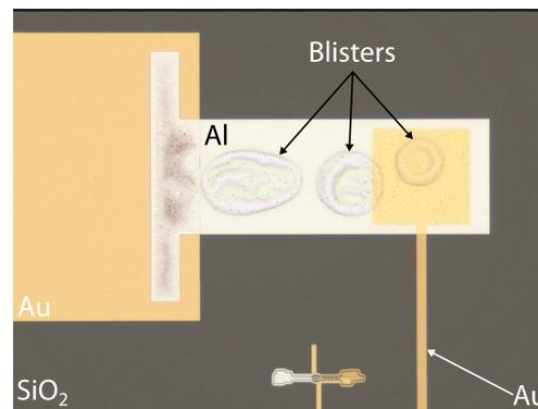
**Figure 5.9:** Plasma-associated aluminum blistering after oxidation.
