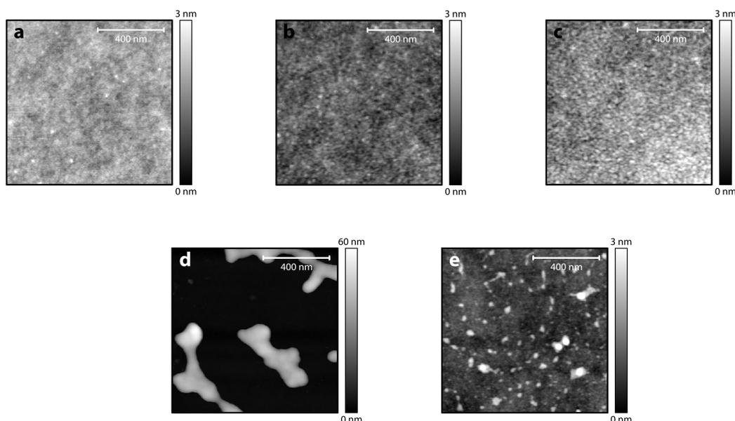
**Figure 4.1:** Morphology of ultrathin COC films after solvent exposure: **a** untreated COC film, **b** COC film after 19 h acetone exposure, **c** COC film after 1 min MIBK exposure, **d** COC film after 1 min anisole exposure, and **e** COC film after 1 min chlorobenzene exposure.
