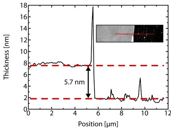
**Figure 4.3:** Determination of thickness of an ultra-thin COC film by AFM. The red solid line represents the line profile.
