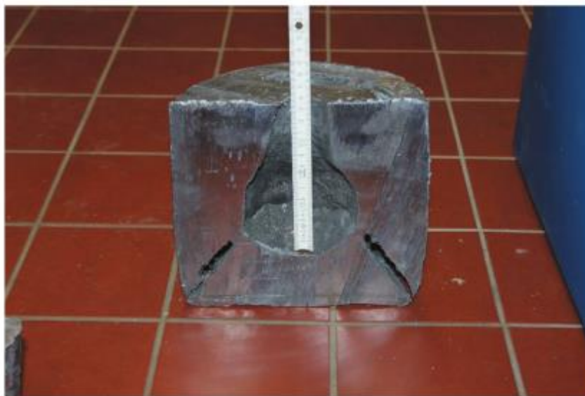
Figure 2. Lead block cut in half after the Trauzl-test.
