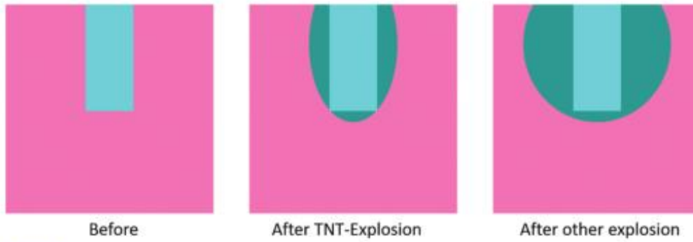
Figure 1. Schematic representation of the Trauzl-test: Lead block (color: Baker-Miller-Pink), cavity filled with explosive (color: turquoise), hole additional to the cavity filled with explosive (color: petroleum green).
