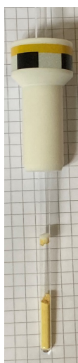
Figure S 9.4-1: NMR sample tube with a PTFE-silicone insert and PI-3-COF sample (yellow). The insert restricts the vapor volume of MeCN to the temperature controlled zone below the spinner.
