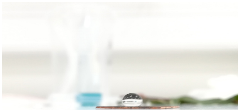
Figure 2.4.9.: Wetting behavior of a modified copper plate reproduced according to Bethke et al. [406]. Contact angle of the superhydrophobic copper plate reaches CAs around 158°.
