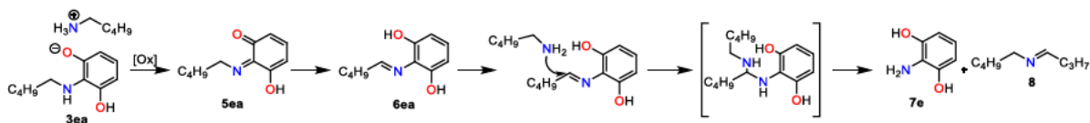
Scheme S9. Proposed mechanism of the step-by-step oxidation/aminolysis of 3ea to 7e .
