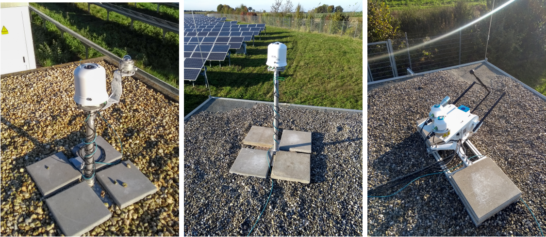
Figure 3.5: ASI-16126 (left), ASI-16142 (middle) and STR-22 (right) as installed on the measurement sites.
