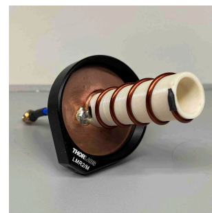
Figure 3.2: Helical antenna used in Ref. [107]
