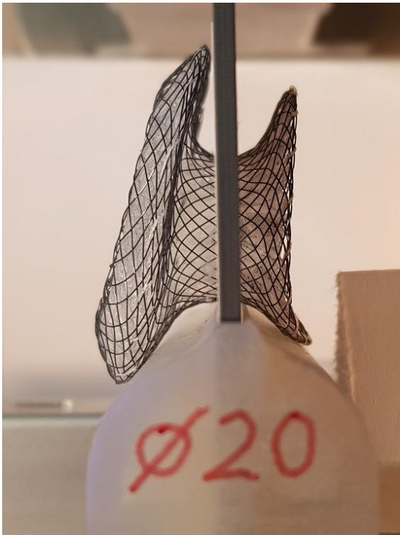
Abbildung 55: ASO 24mm an Septum T=2mm
