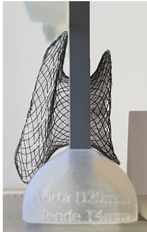
Abbildung 56: ASO 24mm an Septum T=4mm
