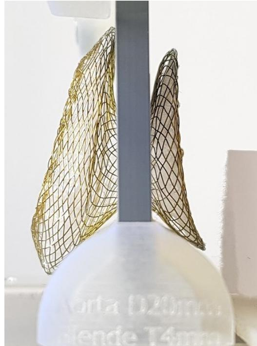
Abbildung 58: FFO 24mm an Septum T=4mm
