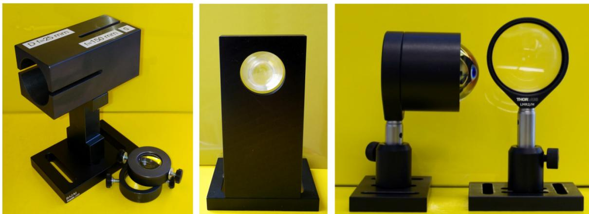
Figure 3-7 Optics used in the QYDS. (left) one inch best form lenses; (middle) one inch Fresnel lens with a focal length of 15 mm; (right) two inch aspheric and plano-convex lens for highest collection efficiency.
