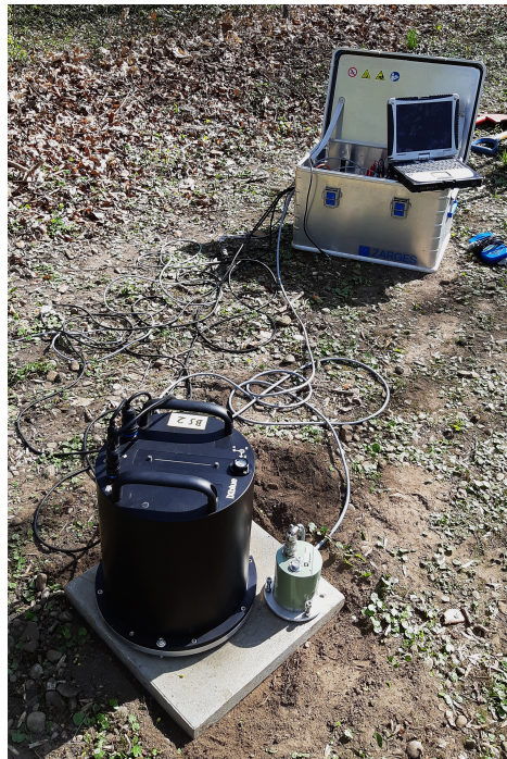
Figure 2.2: Set-up for the single-station six-component noise measurements. The two instruments, the blueSeis-3A rotational sensor on the left and the Trillium Compact 120s seismometer on the right, are placed about 10cm apart on a concrete slab. The instruments are connected to GPS, power and the seismometer to a REFTEK digitizer (inside of metal box). Before starting the recording of the data, a styrofoam insulation box is placed over the instruments
