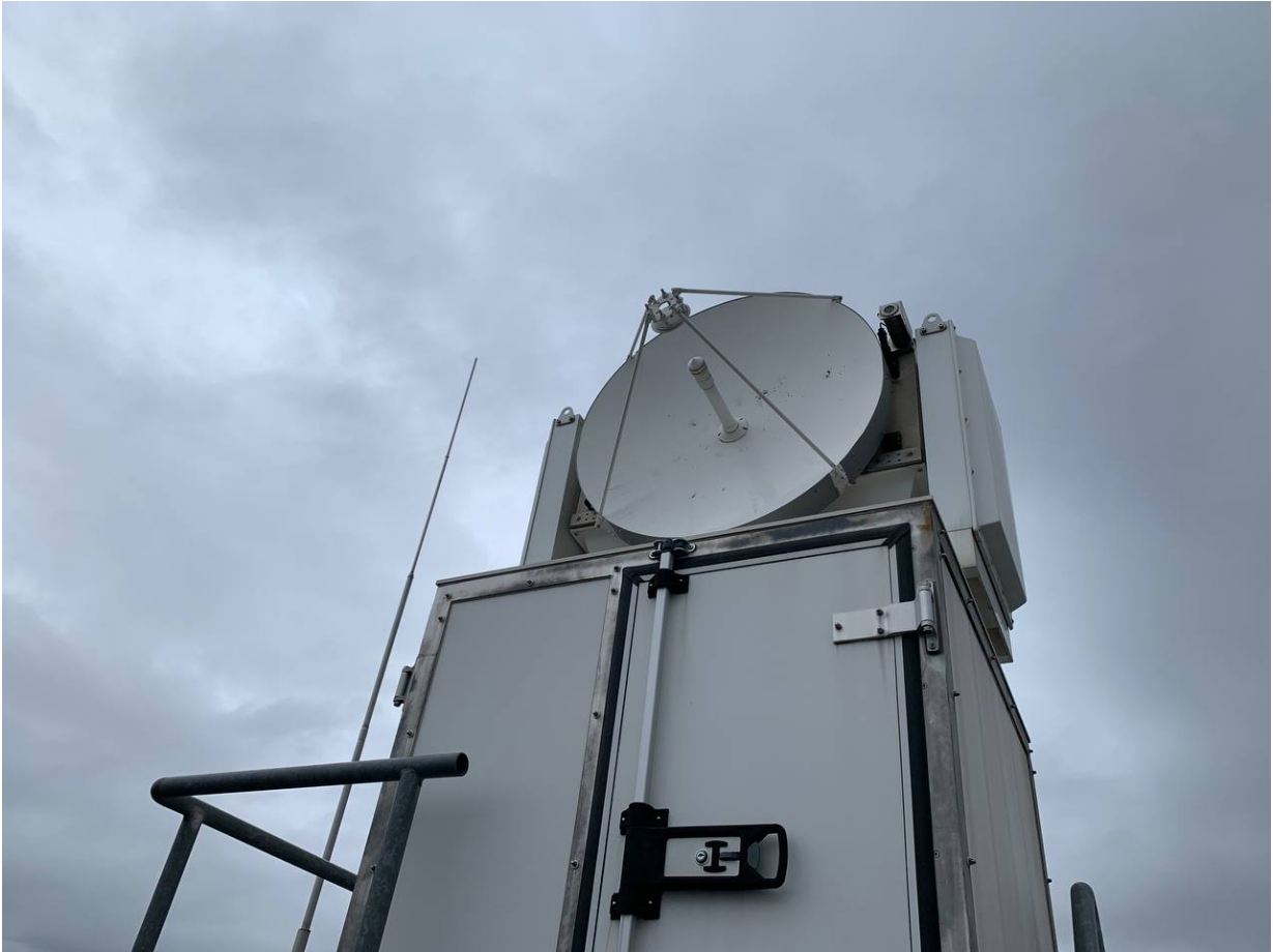
Figure 2.5: MIRA-35 radar, located at the Meteorological Institute Munich (MIM).
