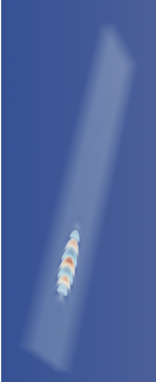
Figure 4.26: Probe-pump collision in a flat-box shaped simulation space in order to detect a polarization rotation of the probe pulse. The probe pulse on the left is tiny in comparison to the strong pump on the right.
