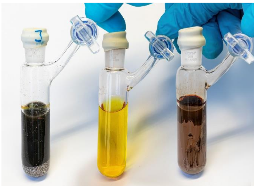
Figure 19. From left to right: (2-Ethylhexyl)sodium ( 36 ) in hexane prepared in batch over metallic sodium, 5 min after addition of 115 . (2-Ethylhexyl)sodium ( 36 ) in hexane prepared via a sodium-packed-bed reactor, 5 min after collecting. (2-Ethylhexyl)sodium ( 36 ) in hexane prepared via a packed-bed sodium reactor, 18 h after collecting.
