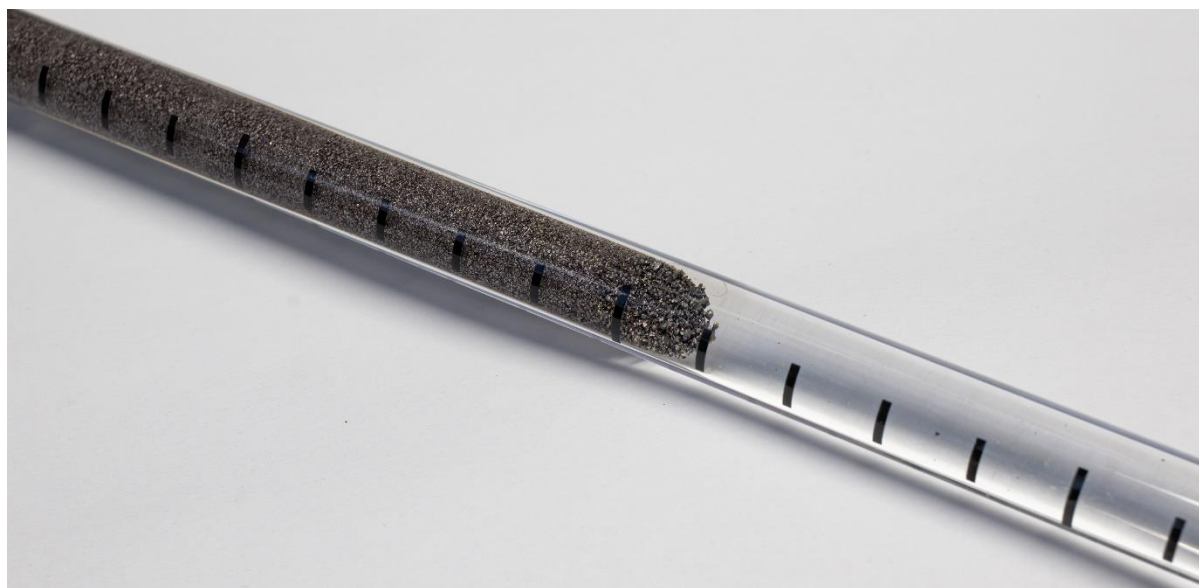
Figure 21: Packed-bed reactor filled with sodium particles of appropriate size.
