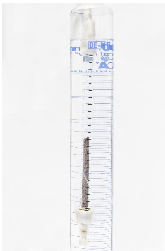
Figure 24: Packed-bed sodium reactor in an i -PrOH bath connected via a nonadjustable endpiece (bottom) to the tubing ( V_{pre1} ) attached to the pump. Adjustable endpiece (top) connected to the tubing ( V_{pre2} ) attached to the T-shaped mixer.
