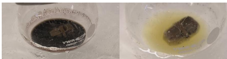
Figure 20: Titration of KDA a) base before titration; b) titration mixture after reaching the endpoint.
