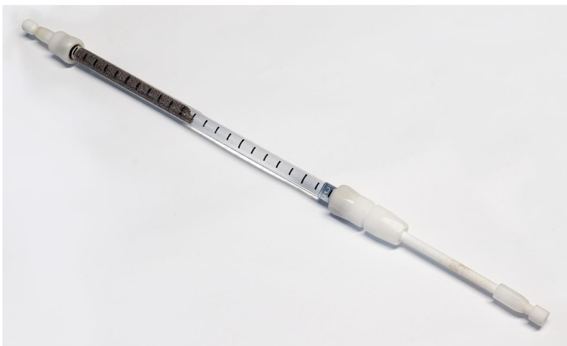
Figure 23: Closed packed-bed reactor filled with sodium particles. Adjustable endpiece set to give the maximum volume of V_{R1} = 7.5 mL.
