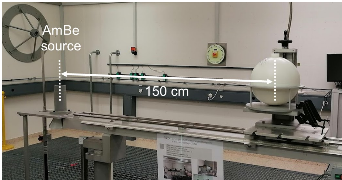
Figure 15: Measurement setup for the calibration of the Passive LINUS.
