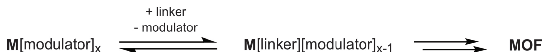
Figure 1.18: Reaction equilibrium during modulated MOF synthesis where the modulator and the linker compete for the coordination on the metal node (M).
