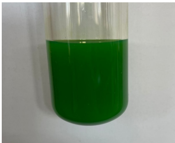
Figure B.19: Green, organic intermediate formed during synthesis from \text{ZrCl}_4 _GB after 1 h reaction indicating that the TCPP linker is protonated to dicationic TCPP ( \text{H}_4\text{TCPP}^{2+} ).
