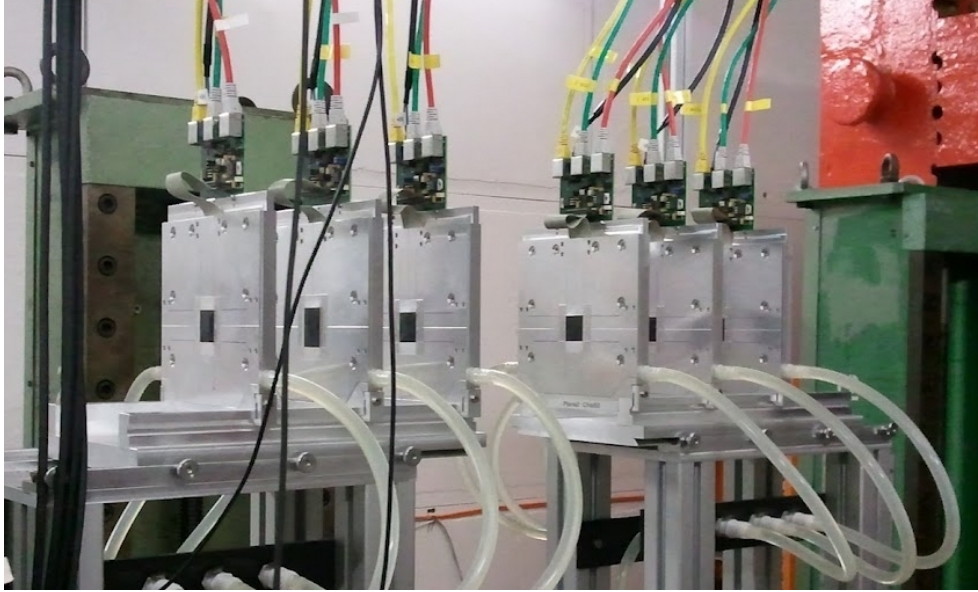
Figure 4.8: The DATURA beam telescope with its sensor planes mounted on aluminium jigs. The boards on the top of each jig provide connections for power, clock, sensor configuration and data transmission. The transparent tubes connected to each jig are used for the water cooling of the sensors.
