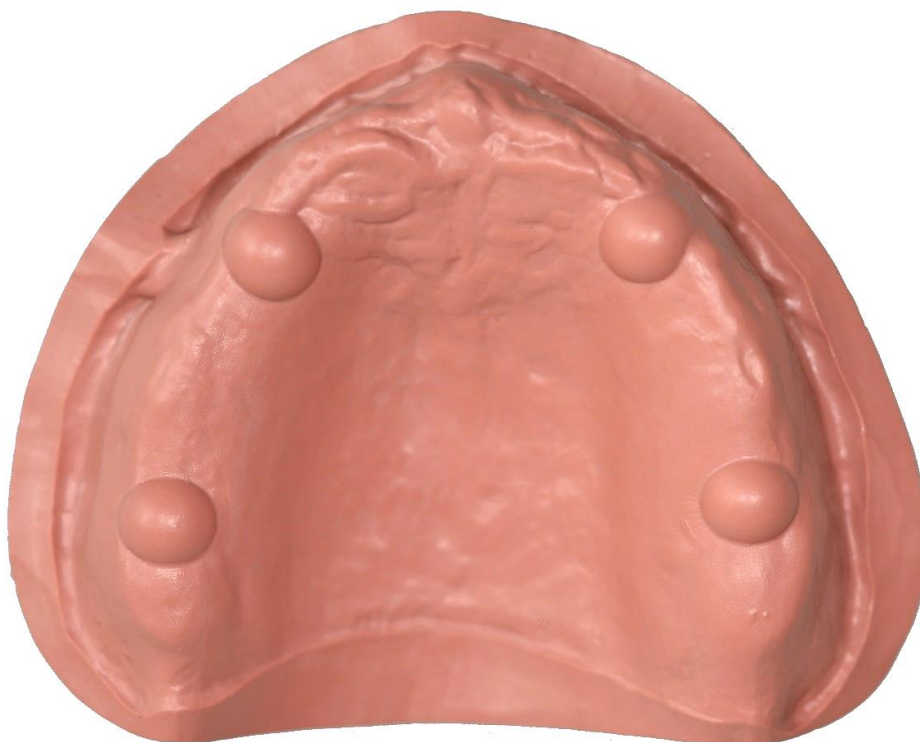
Figure 3.1: Testing model milled from PEEK [119].
