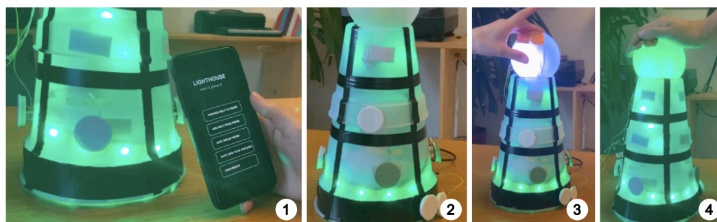
Figure 2.3: Tower technical prototype (1. use app to communicate with other groups; 2. place magnets on the Tower to choose an answer, green means I am confident , white means I am not sure ; 3. rotate top bulb to seek help; 4. touch the top bulb to finish the activity).
