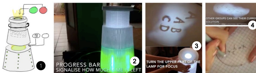
Figure 2.1: stayFOCUSed technical prototype (1. concept idea and structure; 2. show timer with light progress bar; 3. rotate the lamp to show answers; 4. pen-writing on the disk).
