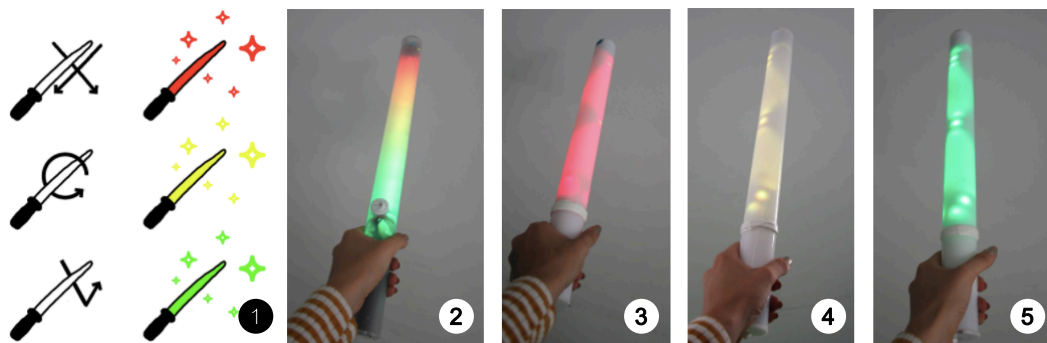
Figure 2.4: Glowing Wand technical prototype (1. different hand gesture designs; 2. switch for a rainbow feedback; 3. negative tick gesture to red light; 4. circle gesture to yellow light; 5. tick gesture to green light).
