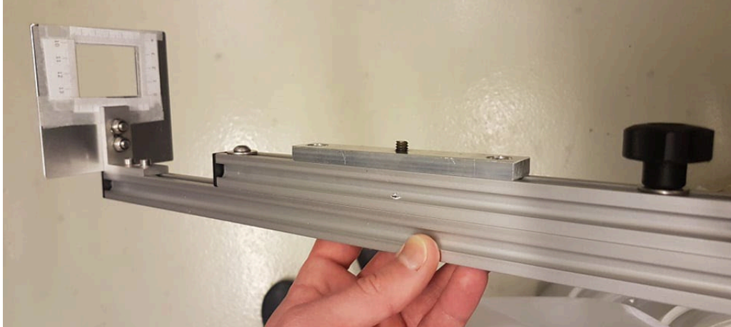
Figure 4.2: Picture of the designed device to ensure always the same distance from camera to the wound.
