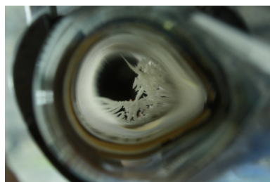
Fig. 3.3: Colourless crystals of BeI 2 are forming at the cooler part of the quartz tube.
