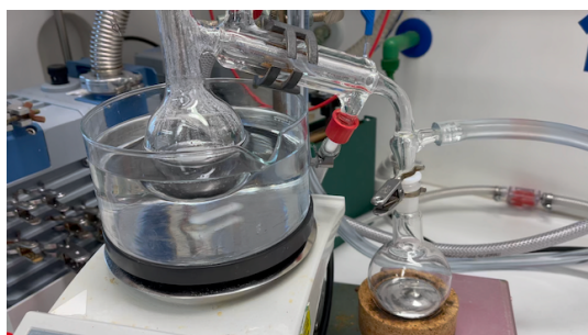
Fig. 3.1: Running distillation of Mercury as performed during the scope of this work.
