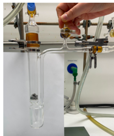
Fig. 7.1: Special Schlenk frit for the separation of liquid and solid components in at elevated temperatures under inert conditions.
