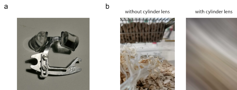
Figure 3.12: Cylinder lens goggles chronically restrict the range of experienced orientations. a) Top view of cylinder lens goggles mounted on a head bar. b) Photo of the home-cage environment without and with a cylinder lens mounted in front of the camera lens.
