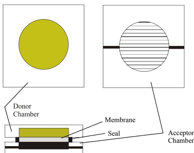
Fig. 3-64 Modified Loth chamber made of acrylic glass for release studies; the donor chamber (left and above) keeps 1.25ml of donor medium at a layer thickness of 4mm; the acceptor chamber (right and top) provided with a ripple plate supporting the membrane is filled with acceptor medium and is connected to the medium reservoir (not shown); chambers are separated by a cellulose acetate filter membrane with 0.45 $\mu$ m pore size; the system is sealed by a polyurethane rubber o-ring;
