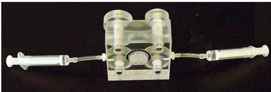
Fig. 3-65 Modified Loth chamber for release studies equipped as static model with two syringes providing the acceptor solution;
