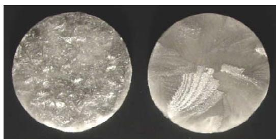
Fig. 3-33 Xerogel pads consisting of hydroxyethyl cellulose 100.000 made from 2.5% hydrogels by conventional freeze drying process without annealing; left: top, right: bottom
