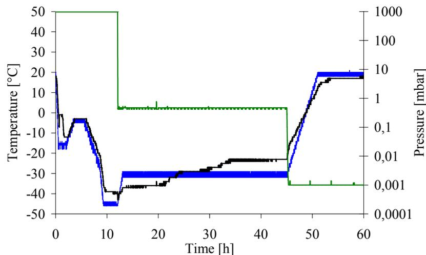
Fig. 3-35 Temperature/pressure – time diagram of freeze drying process with annealing step during freezing; --- plate temperature, --- product temperature, --- cabin pressure
