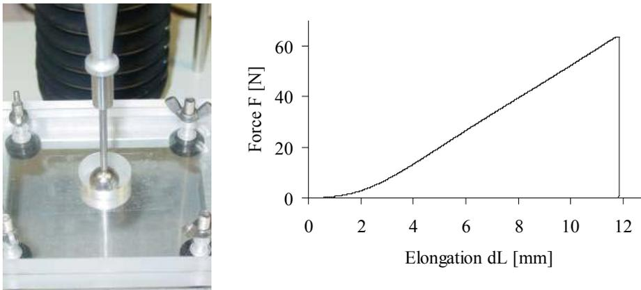
Fig. 3-53 Measurement of elastic modulus with texture analyser (left); force-distance diagram of penetration experiments with rupture at 61.5 N (right);
