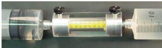
Fig. 3-26 Static mixer with mounting device between two syringes; gel mass is pumped back and forth 10 times for homogenisation;
