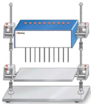
Fig. 2-4 Warm air drier for vials and eppendorf caps;
