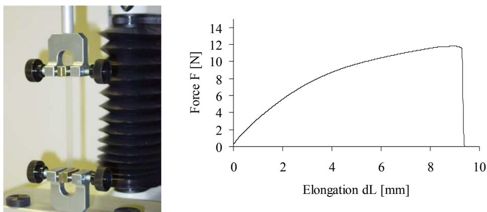
Fig. 3-52 Measurement of tensile strength with texture analyser (left); force-distance diagram of tension experiments with rupture at 11.8 N (right);
