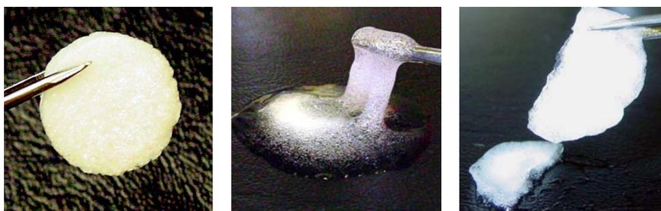
Fig. 3-43 Hydroxyethyl cellulose / gellan gum xerogel pad produced from a hydrogel containing a 2% / 1% mixture of hydroxyethyl cellulose 100.000 and gellan gum F swollen in water; left: dry pad before reconstitution; center: flowing gel pad 5 min after reconstitution with water; right: non flowing gel pad 5 min after reconstitution with isotonic sodium chloride solution;
