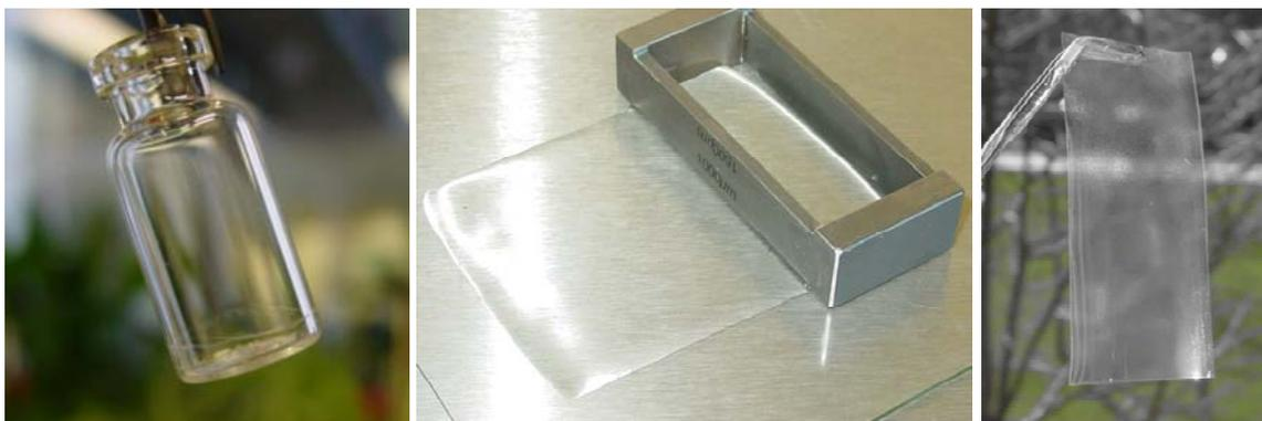
Fig. 3-50 Films made from 2.5% hydroxyethyl cellulose 100.000 hydrogels; left: 2R glass vial with dried film on the bottom and lower side walls; center: wet film being cast out with scraper; right: self-supportive film after removal from plate;
