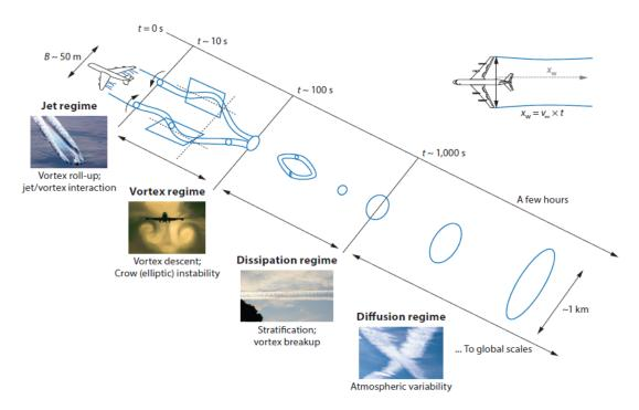
Figure 2.3: Schematic diagram of aircraft wake evolution into four regimes - jet, vortex, dissipation and diffusion. Source: (Paoli and Shariff, 2016)
