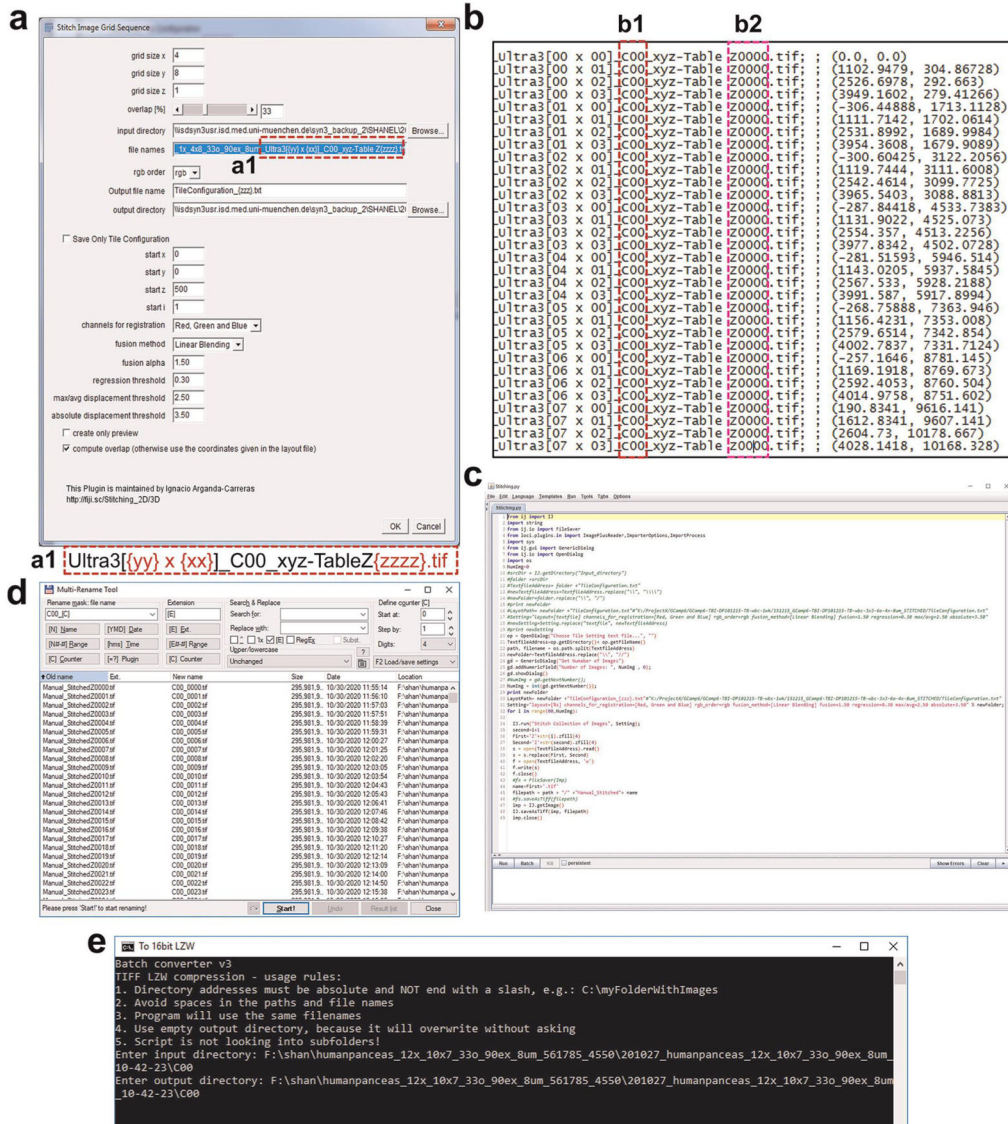
Extended Data Fig. 4 | Key steps for data stitching, renaming and compression. a , One example for correcting information in 'Stitching Image Grid Sequence'; a1 highlights the replacement of red letters in Step 42 about 'file names'. b , The key information of 'TileConfiguration' txt file; b1 highlights the responding channel number that should be corrected and saved in the respective separate folder, and b2 highlights that the starting Z number should be '0000' for all 'TileConfiguration' files. c , The information of 'Stitching.py'. d , One example for settings of 'Multi-Rename Tool'. e , One example of compressing tiff files with 'LZW TIFF'. Panel a produced with software from ref. 50 , Oxford University Press.
