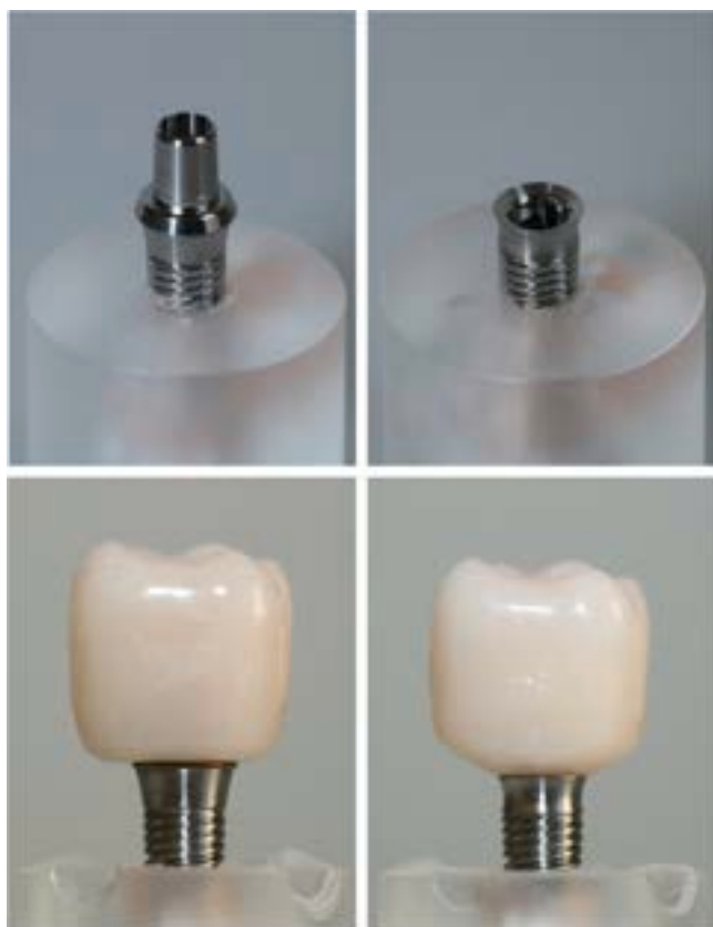
Fig. 2 – Implant type with titanium base (TiB, left) and without (NTiB, right) embedded in acrylic resin showing different interface design.
