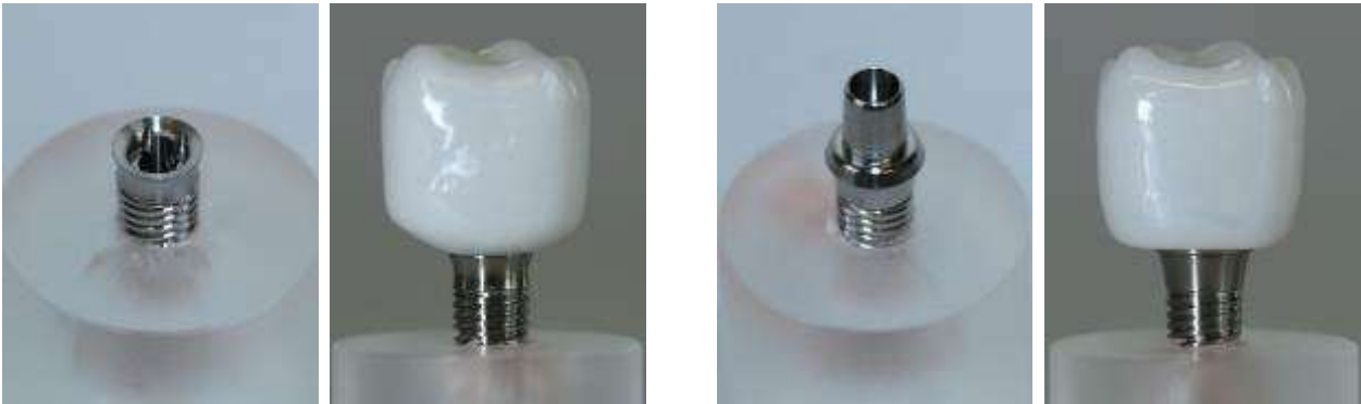
Figure 2: Different interface design of implant type DS (left) and TB (right) embedded in acrylic resin.
