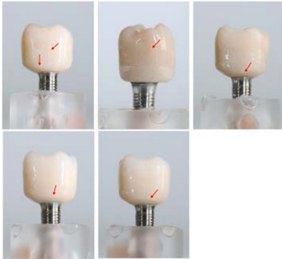
Fig. 5 – Failures during chewing simulation: ND crowns showing cracks (upper), PM crowns showing basal cracks (lower).
