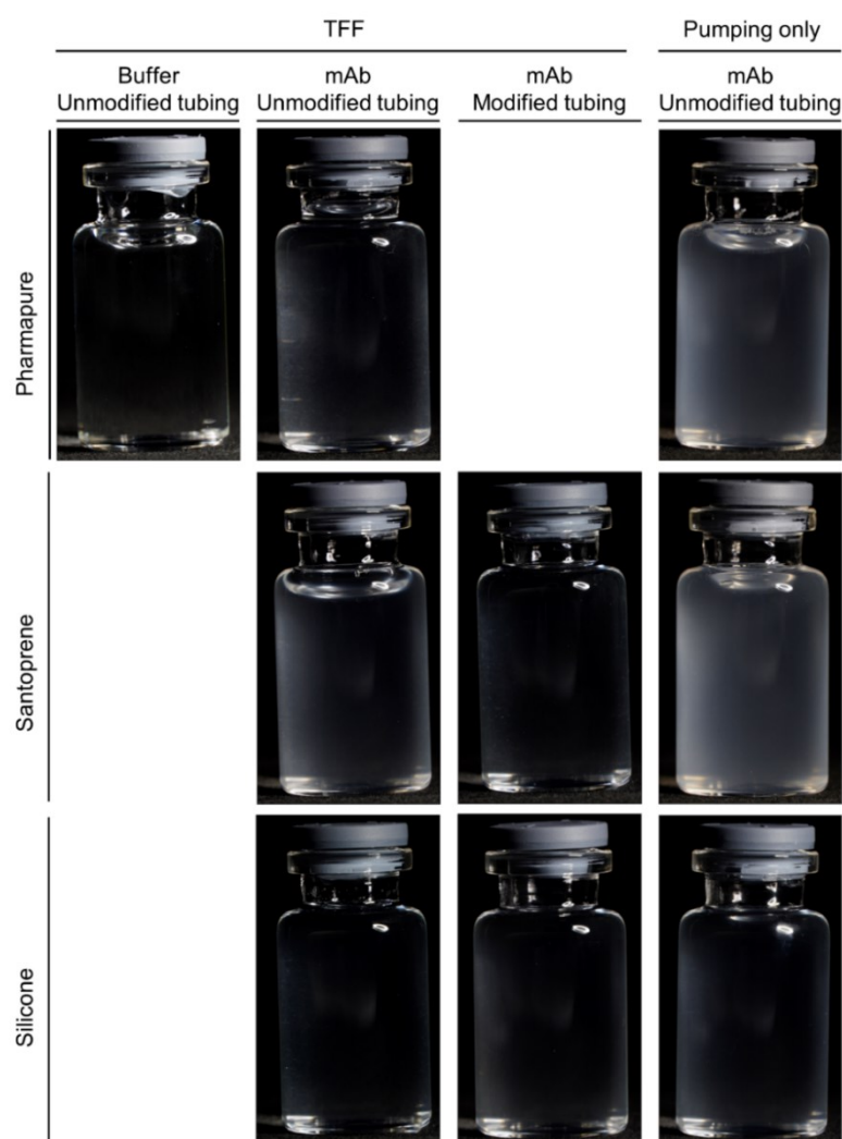
Figure 3 Photo documentation of buffer and mAb samples after diafiltration runs and peristaltic pumping only using different tubings.
