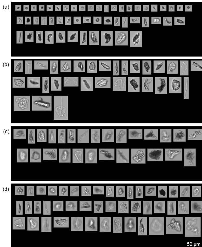
Figure S 2 Exemplary images of particles generated upon pumping pure buffer (a, c) or 1mg/mL mAb (b, d) with (c, d) or without (a, b) addition of 0.01% PS20 in filling mode at 180 rpm.
