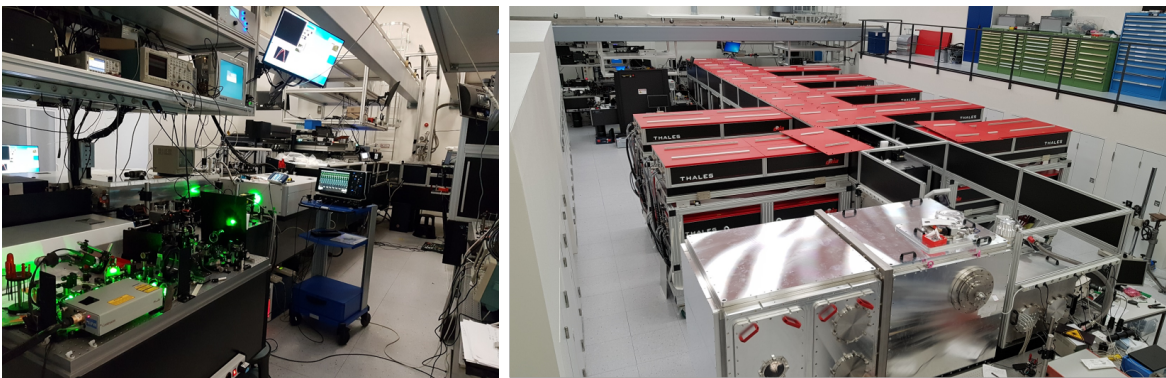
Figure 2.3: ATLAS 3000 hall during the commissioning phase in 2020. The first stages ('front-end') are seen in the left picture. The right picture shows the components and size of the final two amplifiers, which are covered by red lids.
