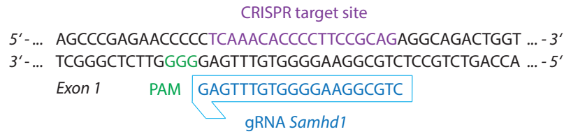
Figure 3.3: Samhd1 gRNA sequence and CRISPR target site for CRISPR/Cas9-mediated KO generation of Samhd1 . The gRNA sequence is indicated in blue, followed by the respective protospacer adjacent motif (PAM) sequence 5'-NGG-3' indicated in green and the CRISPR target site indicated in purple. The gRNA used for Samhd1 in this study binds at the beginning of the Samhd1 gene in Exon 1.
