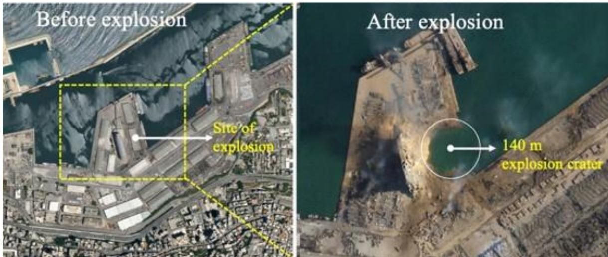
**Figure 8.** Harbour of Beirut before and after the accident in 2020, caused by improperly stored ammonium nitrate.
