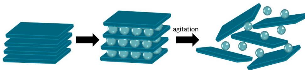
Fig. 1.2 Schematic description of the redox-mediated exfoliation approach. The layers are depicted in cyan, while the oxidizing or reducing agent is given as turquoise spheres. By treating the layered material with an oxidizing or reducing agent, the properties of the interlayer space are modified, and the following agitation enables the delamination of the layered material.
