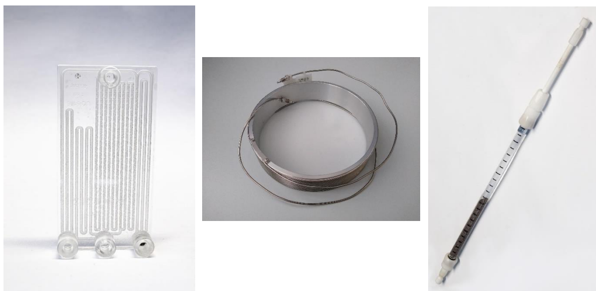
Figure 2. Pictures of chip (picture taken by Peter Dowling), coil and packed-bed reactors (picture taken by Johannes H. Harenberg).
