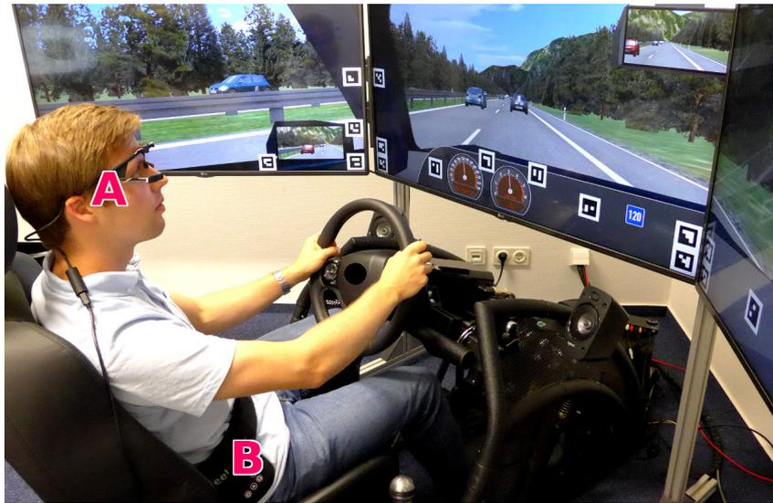
(a) Setup showing the driving simulator, eye-tracker (A), vibrotactile belt as LLI (B), and the driving scene from Figure 5.2 (T1).
