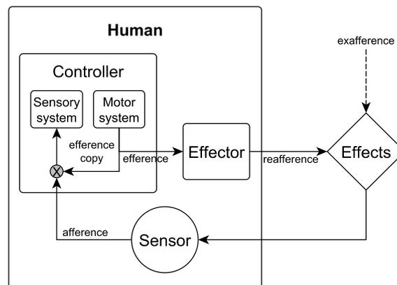
Figure 4.1: Illustration of the refference principle within an expanded diagram for a human sensorimotor feedback loop (see Figure 3.2a).
