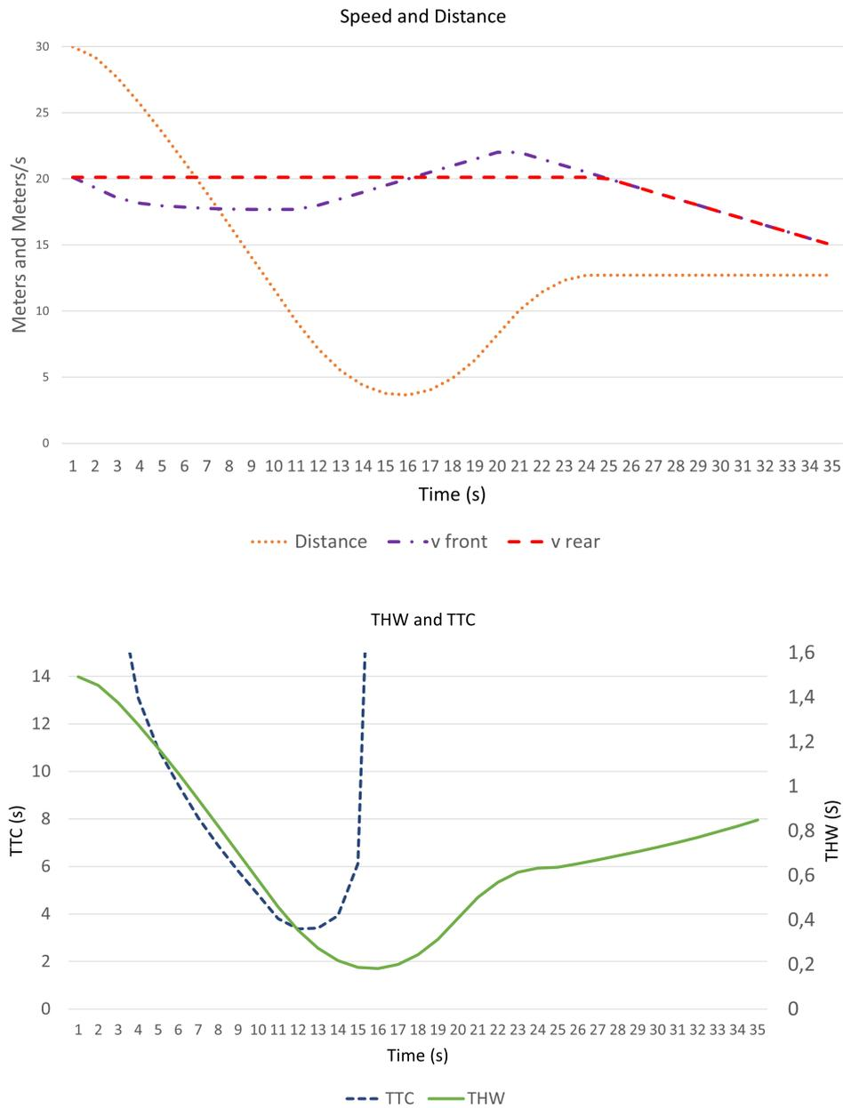
Figure 2.3: Top: Distance (orange) between two vehicles driving on the same lane as a function of each vehicle's speed (red, purple). Bottom: THW (green) and TTC (blue) for the same scenario.
