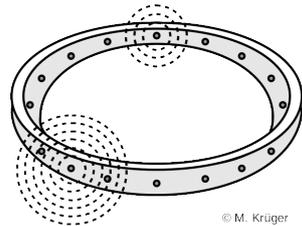
(b) Sketch of the tactile interface with two active vibromotors (out of 16).
