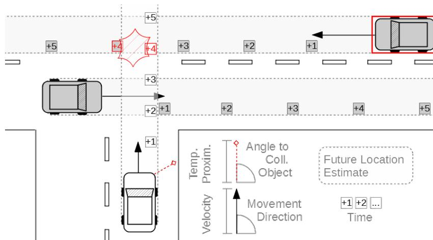
Figure 6.1: Illustration of the TTC estimation procedure with two spatial dimensions. Predicted trajectories are annotated with time markers that indicate the predicted vehicle's front position at the respective time. Arrows represent the moving direction (angle) and velocity (length). Vehicles with a predicted collision (spatial and temporal overlap) are highlighted.
