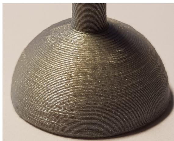
**Figure 5.** Single printed layers of a 3D printed object
