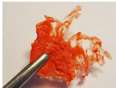
Figure 9. Precipitate 1 - Polybutadiene
