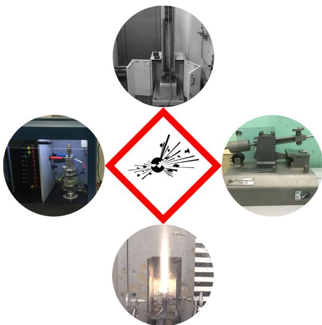
**Figure 7:** Clockwise from top: Impact sensitivity test, friction sensitivity test, steel-sleeve test, and ESD test.
