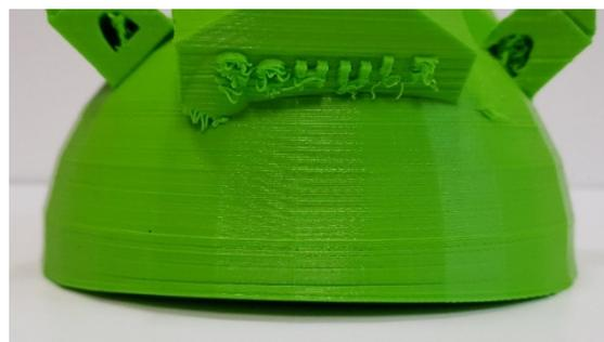
**Figure 6.** The Warp effect is clearly recognizable on the bottom side of this object made of ABS
