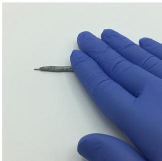
**Figure 4:** The sparkler is formed by rolling the mixture by hand.
