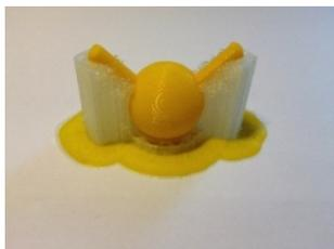
**Figure 12.** "Sulfur atom" made of PLA with supporting structure of PVA
