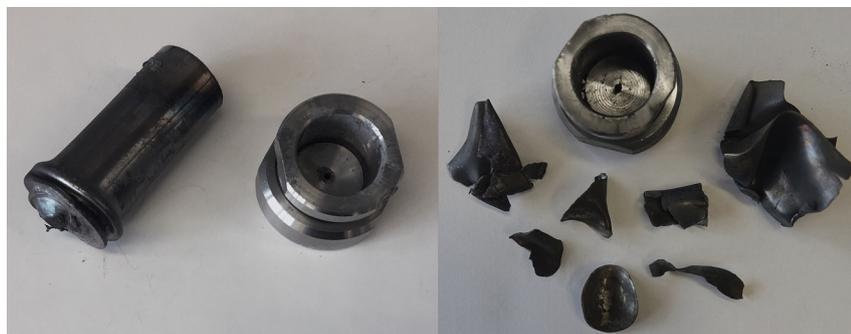
**Figure 8:** Left: Although the steel sleeve used in the steel-sleeve test with the self-made sparklers is deformed at the bottom, the test can still be considered negative. Right: The steel sleeve of a steel-sleeve test used for the bought sparklers was blown up into seven parts. Thus, the steel-sleeve test was not passed.
