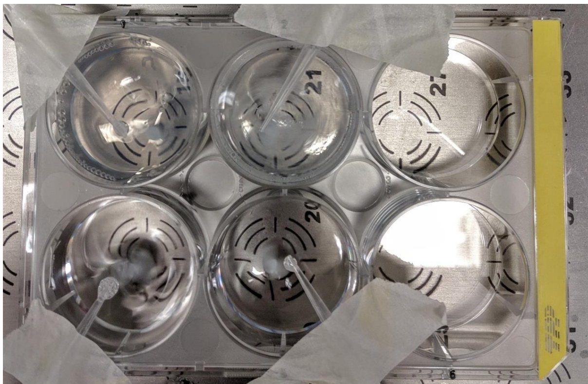
Figure 3: Preparation of alginate nanoparticles in a 6-well plate. The protein- \text{CaCl}_2 mixture was added dropwise and caused turbidity of the solution.
