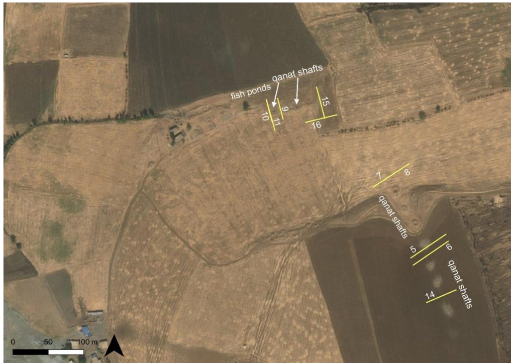
Figure 5.4. Bing satellite image of the southeastern area of the Bora Plain where the openings of qanat shafts are still visible today. The yellow lines show the positions of the ERT profiles (note that profiles 10-11 and 7-8 were very close to one another so they appear as a single line in the image). The label “fish ponds” shows the location of fish ponds that were created after the satellite image had been taken; they were already in use in 2015 when PPP started work in the region. Prepared by Andrea Squitieri.
