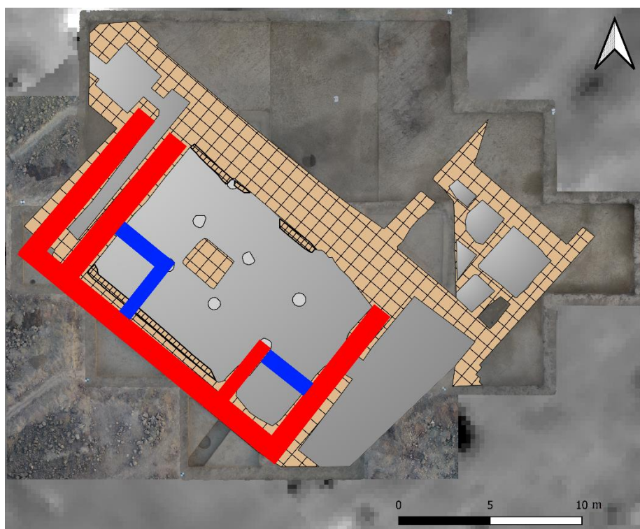
Figure 2.5. Interpretation based on ERT results overlapped on the reconstruction of the structure. The red lines illustrate the walls detected in both ERT results and the excavation and the blue lines show the walls observed by ERT results and not in the excavation.
