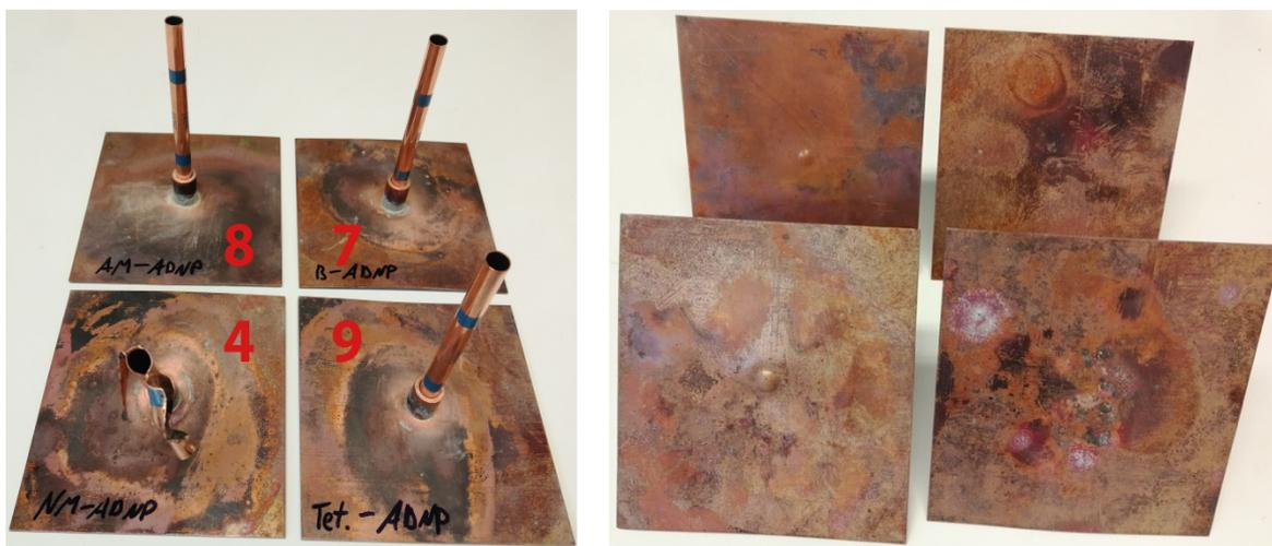
**Figure 46.** Negative test results using neat lead azide (left) and bottom of the respective witness plates (right).
