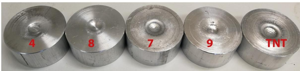
Figure 44. Aluminum witness blocks and indentation caused by the respective compound (4, 7, 8, 9).
