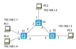
Figure 63: Topology *topo3*. The numbers around a switch indicate the ports from which it connects to other switches or end-points.
