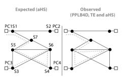
Figure 42: An example of the distributed conflict class *policy suppression by upstream traffic looping*, observed when deploying together the control applications Destination-based Path Load Balancer (PPLB4D), Traffic Engineering (TE) and active Host Shadowing (aHS)
