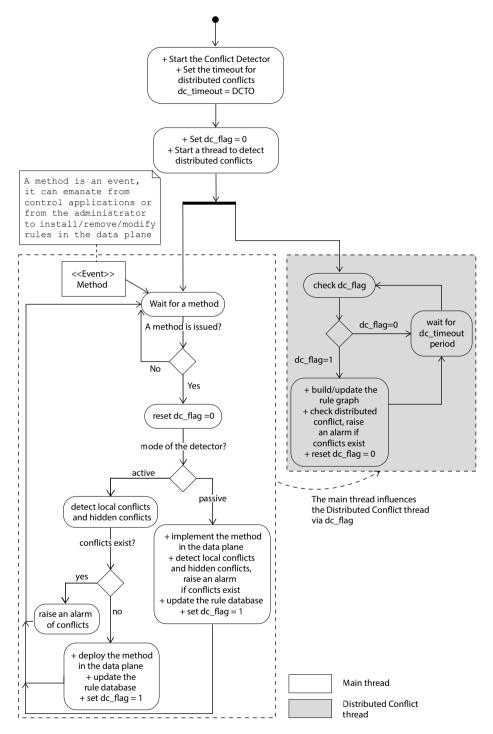
Figure 69: The mechanics of the conflict detector. The Distributed Conflict thread is meant to detect distributed conflicts, in our case it targets the general traffic looping and traffic dropping. Reyes [90] implements the detection of conflicts related to packet modification also in this thread.
