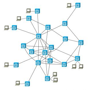
Figure 22: A random topology generated with the Barabasi-Albert model [4] (20 switches, 10 end-points, reproduced from Reyes' work [90])
