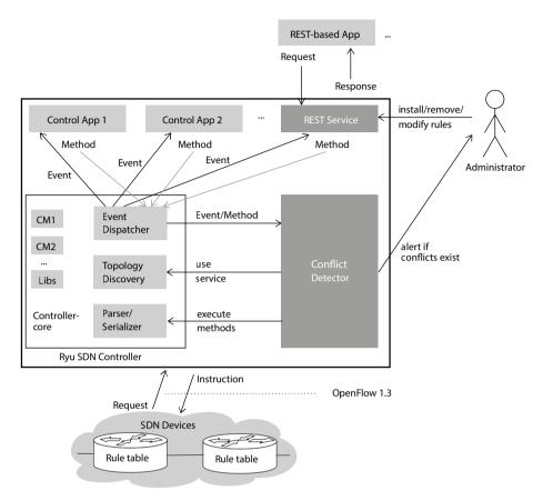
Figure 67: Communication of the conflict detector with other controller modules (CM) of the Ryu SDN framework. The *Conflict Detector* and *REST Service* boxes are our added components.
