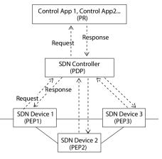
Figure 12: A possible mapping of the SDN architecture to the PCIM model
