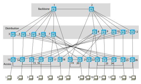
Figure 71: The simulated topology for the Stanford's backbone network [50]
