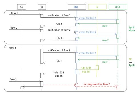
Figure 49: An example of a hidden conflict observed when co-deploying the End-point Load Balancer (EpLB), Traffic Engineering (TE) and Shortest Path First Routing (SPF) control applications, observed in experiment 6 in Chapter 3.6.3. S6, S7 are switches in the data plane, Ctrl is the controller. The match fields of rule 1 cover only traffic flow 1, of rule 2 only traffic flow 2, and of rule 1234 both. Rule 1234 has lower priority than rule 1 and rule 2.
