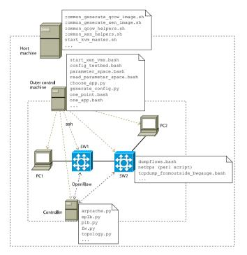
Figure 25: Illustration of a simple test-bed with the associated programs in each class of machines
