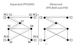
Figure 43: An example of the distributed conflict class *policy suppression by downstream traffic dropping*, observed when deploying together the control applications Destination-based Path Load Balancer (PPLB4D) and Firewall (FW) (reproduced from experiment 4 in Chapter 3.6.3)
