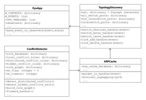
Figure 68: The class diagram of the conflict detector. The visibility of the classes' attributes and operations accords with the UML conventions, i.e., +: *public*, -: *private*, #: *protected*.
