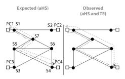
Figure 48: A subtle case of the distributed conflict class *policy suppression by changes to paths*, observed when co-deploying the active Host Shadowing (aHS) and Traffic Engineering (TE) control applications
