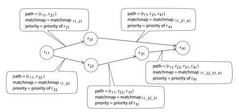
Figure 59: Illustration of edge attributes in a simple rule graph
