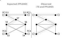
Figure 52: An example of the hidden conflict class event suppression by changes to paths, observed when deploying together the control applications Traffic Engineering (TE) and Destination-based Passive Path Load Balancer (PPLB4D)
