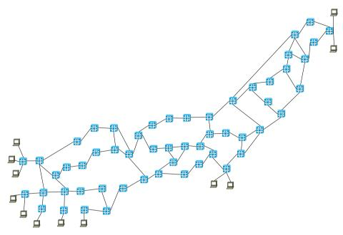
Figure 21: A designed topology simulating the core backbone of the Nippon Telegraph and Telephone (NTT) network [1] in Japan (55 switches, 12 end-points, reproduced from Reyes' work [90])
