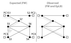
Figure 46: An example of the distributed conflict class *policy suppression by upstream packet modification*, observed when co-deploying Firewall (FW) and End-point Load Balancer (EpLB)
