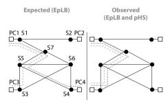
Figure 45: An example of the distributed conflict class policy suppression by downstream packet modification, observed when co-deploying the End-point Load Balancer (EpLB) and passive Host Shadowing (pHS) control applications
