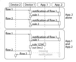
Figure 7: Interactions of an application in isolation and when conflicting with another [25]. For clarity, the controller intermediary has been omitted.
