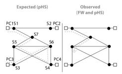
Figure 51: An example of the hidden conflict class event suppression by upstream traffic dropping, observed when deploying together the control applications Firewall (FW) and passive Host Shadowing (pHS)
