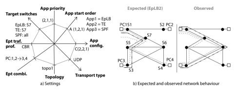
Figure 32: Experiment 6: settings, expected and observed network behaviour
