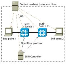
Figure 24: Illustration of a simple test-bed for a network containing two end-points and two SDN devices
