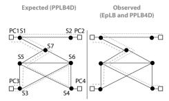
Figure 53: An example of the hidden conflict class action suppression by packet modification, observed when deploying together the control applications End-point Load Balancer (EpLB) and Destination-based Passive Path Load Balancer (PPLB4D)
