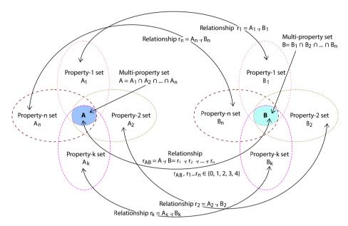
Figure 56: The relationship of two multi-property sets A and B, denoted as  $r_{AB} = A \cdot_r B$ , is calculated by combining all individual relationships of their associated single-property sets  $r_1 = A_1 \cdot_r B_1$ ,  $r_2 = A_2 \cdot_r B_2$ ,  $\cdots r_n = A_n \cdot_r B_n$ . The relationship combination operator is denoted as  $\cdot r$  (pronounced as "dot r").
