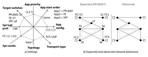
Figure 29: Experiment 3: settings, expected and observed network behaviour
