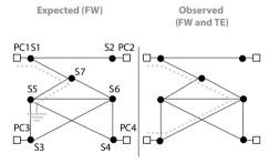
Figure 47: An example of the distributed conflict class *policy suppression by changes to paths*, observed when co-deploying the Firewall (FW) and Traffic Engineering (TE) control applications
