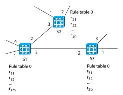
Figure 57: A network part containing three switches S1, S2 and S3. The numbers around a switch indicate the ports from which it connects to other switches or end-points.
