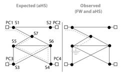
Figure 44: An example of the distributed conflict class *policy suppression by upstream traffic dropping*, observed when deploying together the control applications Firewall (FW) and active Host Shadowing (aHS)
