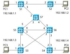
Figure 26: Topology *topo1* for the experiments. The numbers surrounding a switch indicate its port names.
