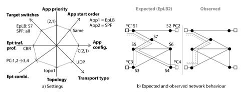
Figure 31: Experiment 5: settings, expected and observed network behaviour
