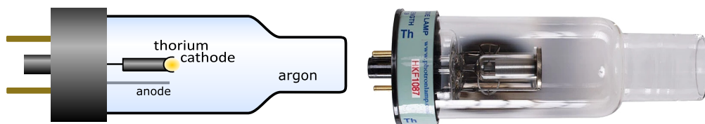
Fig. 2.15.: Illustration of a ThAr hollow cathode lamp, similar to the one that is installed inside the calibration unit of FOCES . Right image is taken from Photron : https://www.photronlamp.com/ on the 14.3.2021 at 14:40.
